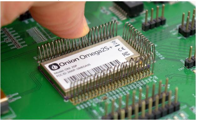
Refer to our visual guide for more clarity on the combing procedure: <a href="https://youtu.be/aoYadArVJPw">https://youtu.be/aoYadArVJPw</a>  Always check that each rail-pin is connected to its corresponding Omega castellated socket before powering the device. The image below represents the incorrect positioning of the rail-pin:
