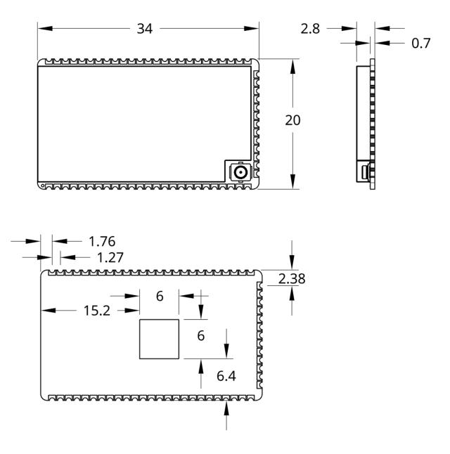
\* All measurements in millimeters
