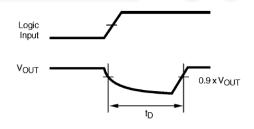
Figure 6. Break-Before-Make Interval Timing
