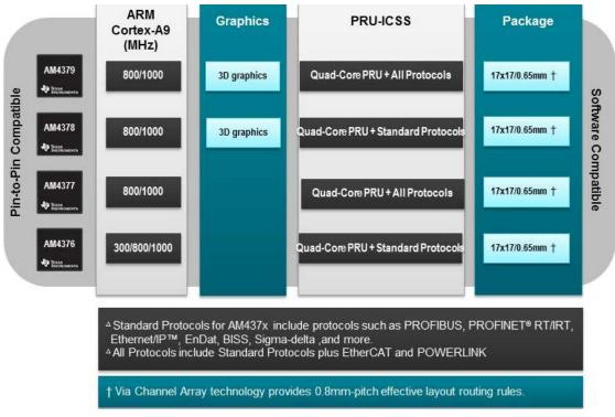
Figure 1-3 AM437x Devices Comparison
