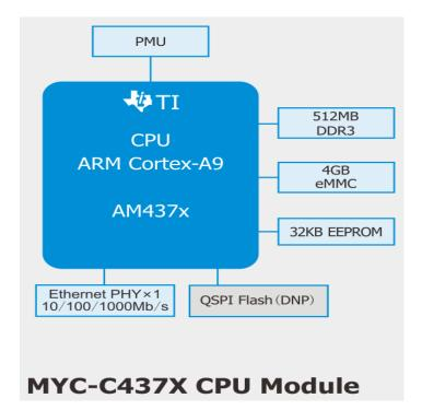
Figure 1-8 MYC-C437X Function Block Diagram
