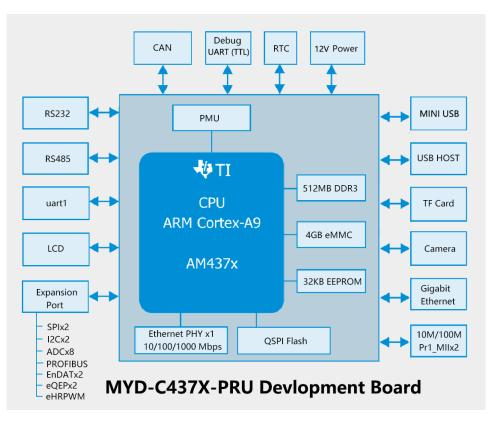
Figure 1-9 Function Block Diagram of MYD-C437X-PRU
