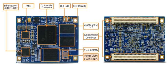
Figure 1-6 MYC-C437X CPU Module
