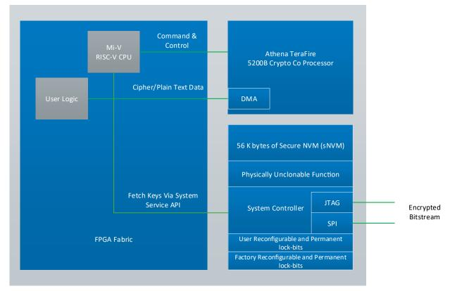
Users instantiate a RISC-V CPU for command and control, including fetching keys from the system controller through a system service API, initializing the Athena Core, and setting up DMA to perform the desired function. The TeraFire core comes with a complete firmware driver library for all supported protocols. These driver libraries are delivered to the designer's desktop through our Firmware Catalog within Libero SoC PolarFire.
