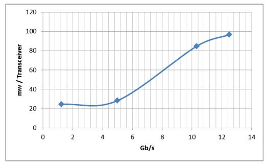
Figure 11-1. Transceiver Power versus Data Rate
