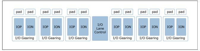
The number of I/O pins varies depending on the device and package size. The persistent I/O feature preserves a state on an I/O without user intervention during programming mode. The PolarFire FPGA I/O buffers are constructed from the following main sub modules.
