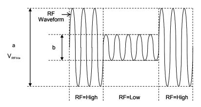
The RF waveform is measured with a calibration coil specified in ISO/IEC 10373-6.
