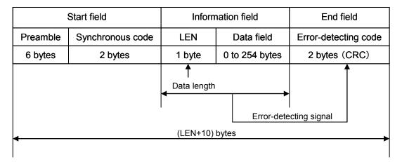
Figure 4-2 JISX6319-4 Frame Format
