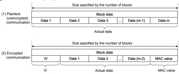
Figure 4-12 Block Data Structure
