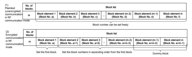
Figure 4-11 Block List Referenced from this RFID
