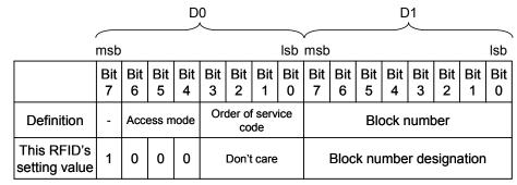
Figure 4-9 Block Element of 2 Bytes
