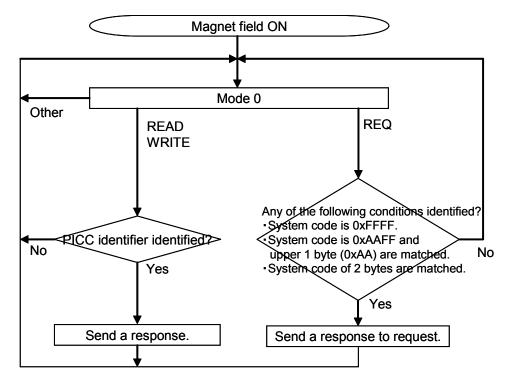
Figure 4-4 JISX6319-4 Flow Chart of Command Processing
