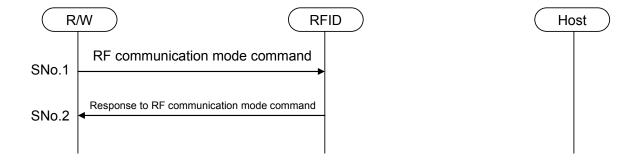
Figure 4-1 RF Communication Mode Sequence
