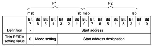
Figure 4-26 Address Specification
