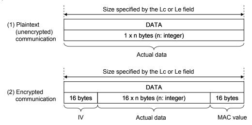
Figure 4-27 Data Block Structure
