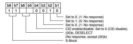
Figure 4-18 S-block Coding
