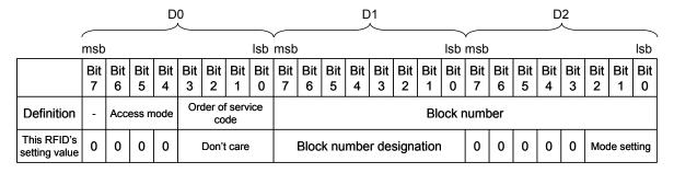
Figure 4-10 Block Element of 3 Bytes
