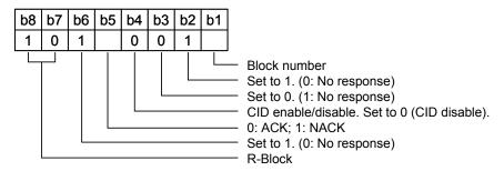
Figure 4-17 R-block Coding
