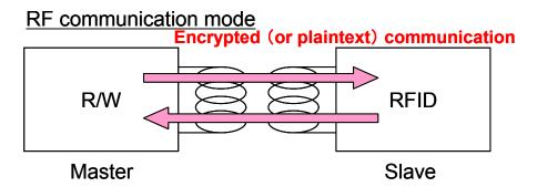
Figure 1-3 Encrypted Communication Function
