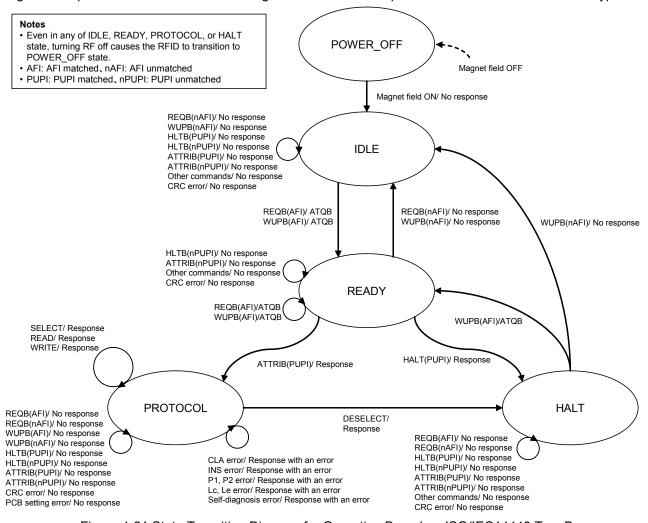
Figure 4-21 State Transition Diagram for Operation Based on ISO/IEC14443 TypeB
