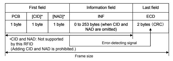
Figure 4-15 ISO/IEC14443-4 Block Format
