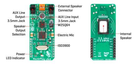
To allow the out-of-box functionality, the Click board<sup>TM</sup> is equipped with a small omnidirectional electret microphone, along with a miniature  $8\Omega$  speaker.
