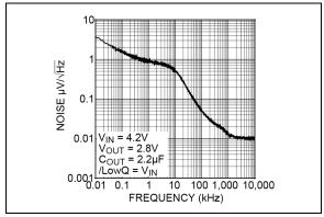
FIGURE 2-22: LDO2 Output Noise Spectral Density.
