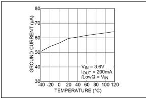
FIGURE 2-19: LDO2 Ground Current vs. Temperature.
