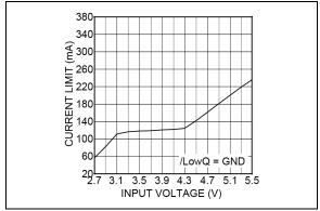
**FIGURE 2-10:** Current Limit vs. Input Voltage.
