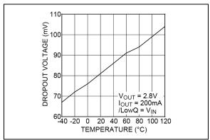
**FIGURE 2-21:** LDO2 Dropout Voltage vs. Temperature.
