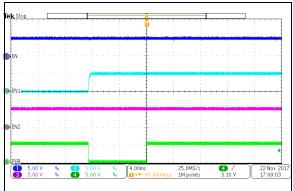
FIGURE 2-31: POR Behavior; EN = EN2 = High, Low-to-High Transition on EN1.
