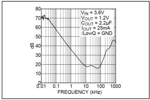
**FIGURE 2-12:** Power Supply Rejection Ratio LDO1 (LOWQ Mode).
