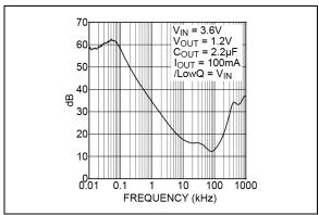
FIGURE 2-13: Power Supply Rejection Ratio LDO1 (Normal Mode).
