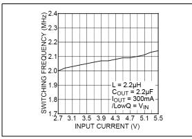
**FIGURE 2-2:** Switching Frequency vs. Input Voltage.
