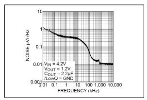
**FIGURE 2-11:** Output Noise Spectral Density.
