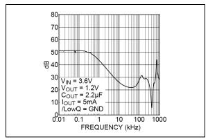
**FIGURE 2-7:** Power Supply Rejection Ratio.
