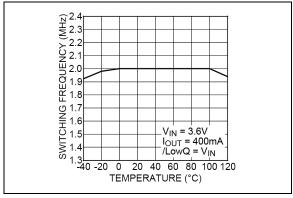
**FIGURE 2-3:** Switching Frequency vs. Temperature.
