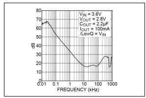
**FIGURE 2-16:** Power Supply Rejection Ratio LDO2 (Normal Mode).
