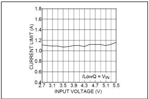
FIGURE 2-6: Current Limit vs. Input Voltage.
