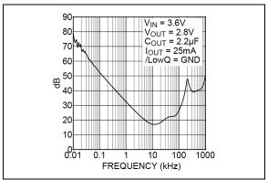
**FIGURE 2-15:** Power Supply Rejection Ratio LDO2 (LOWQ Mode).
