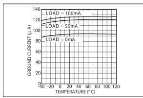
**FIGURE 2-3:** Ground Current vs. Temperature for LDO 3.
