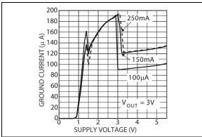
FIGURE 2-25: Ground Current vs. Supply Voltage for LDO 3.
