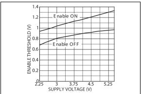
FIGURE 2-12: Enable Threshold vs. Supply Voltage for LDO 3.
