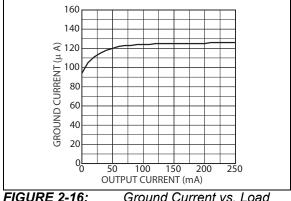
FIGURE 2-16: Ground Current vs. Load Current for LDO 3.
