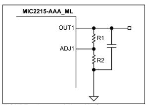
FIGURE 5-1: Adjustable Output.
