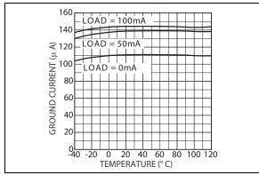
**FIGURE 2-1:** Ground Current vs. Temperature for LDO 1.
