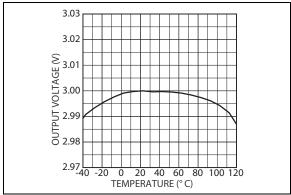
FIGURE 2-6: Output Voltage vs. Temperature for LDO 3.
