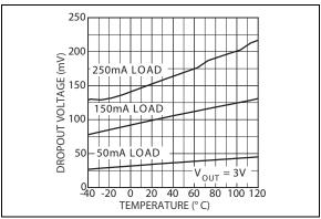
FIGURE 2-7: Dropout Voltage vs. Temperature for LDO 1.
