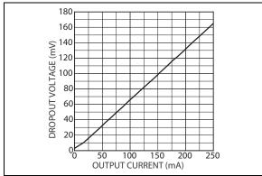
FIGURE 2-20: Dropout Voltage vs. Output Current for LDO 1.
