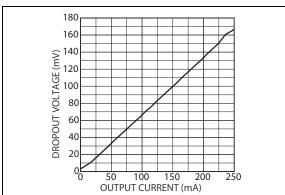
FIGURE 2-21: Dropout Voltage vs. Output Current for LDO 2.
