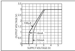
FIGURE 2-26: Output Voltage vs. Supply Voltage for LDO 1.
