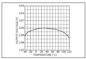
**FIGURE 2-4:** Output Voltage vs. Temperature for LDO 1.
