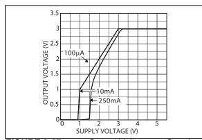
FIGURE 2-27: Output Voltage vs. Supply Voltage for LDO 2.
