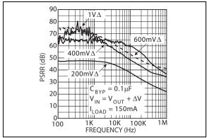
**FIGURE 2-29:** Power Supply Rejection Ratio, 3V<sub>OUT</sub>.
