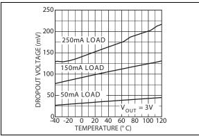
FIGURE 2-8: Dropout Voltage vs. Temperature for LDO 2.
