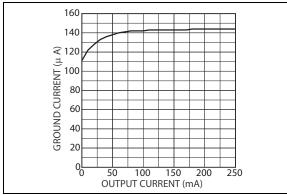
FIGURE 2-14: Ground Current vs. Load Current for LDO 1.
