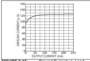
FIGURE 2-15: Ground Current vs. Load Current for LDO 2.
