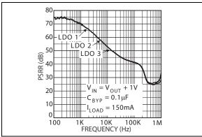
FIGURE 2-31: Power Supply Rejection Ratio.
