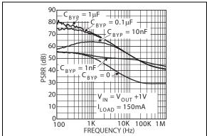
FIGURE 2-30: Power Supply Rejection Ratio vs. C<sub>BYPASS</sub>.
