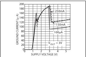
FIGURE 2-24: Ground Current vs. Supply Voltage for LDO 2.
