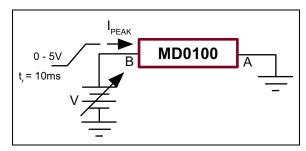
FIGURE 3-8: Test Setup for I<sub>PEAK</sub>.
