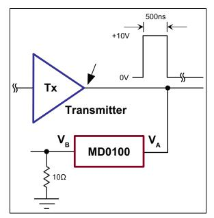
**FIGURE 3-2:** Test Setup for  $T_{OFF}$ .
