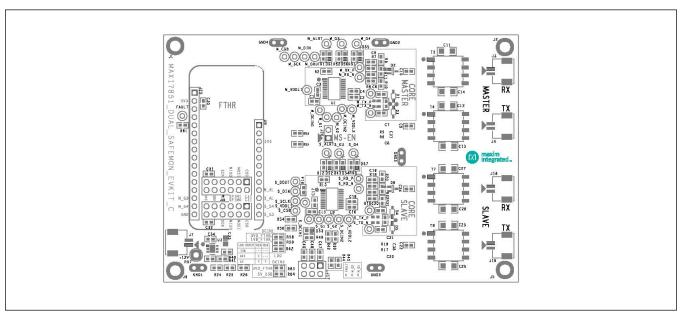
Figure 28. Layout Example: Top Layer Silkscreen
