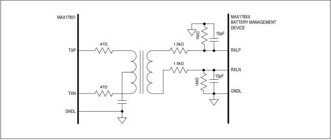
Figure 24. Transformer Coupling of UART Signals
