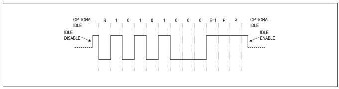
Figure 13. UART Timing for a Preamble
