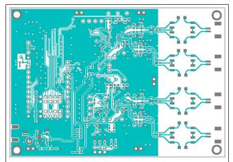
Figure 30. Layout Example: Top Metal
