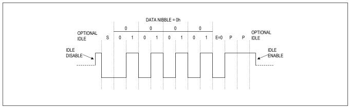
Figure 15. UART Timing for a Manchester-Encoded Data Nibble 0h
