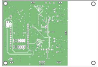
Figure 33. Layout Example: Layer Three Metal
