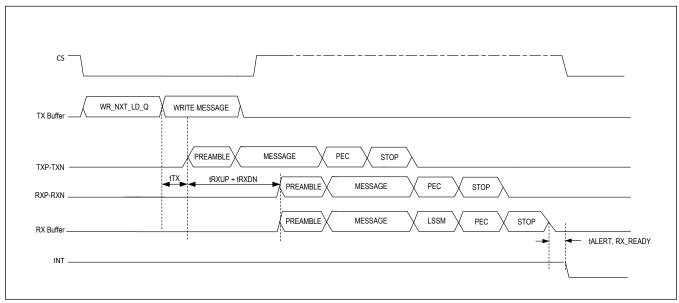
Figure 4. TX Buffer Write and Read
