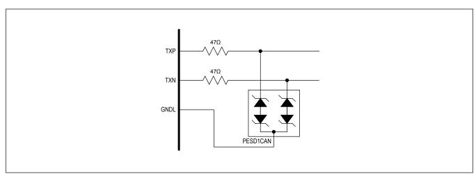
Figure 25. Supplemental ESD Protection for UART Transmitter
