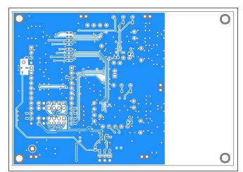
Figure 32. Layout Example: Bottom Metal
