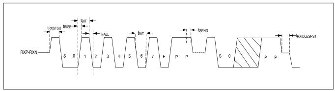
Figure 2. Receive UART Timing
