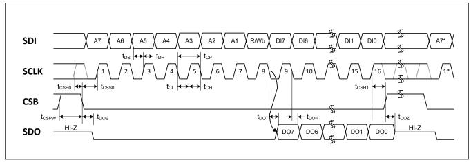
Figure 1. SPI Timing Diagram
