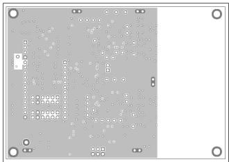
Figure 31. Layout Example: Layer Two Metal
