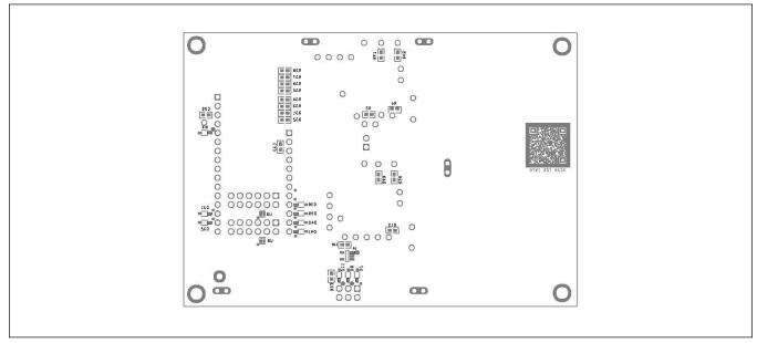
Figure 29. Layout Example: Bottom Layer Silkscreen
