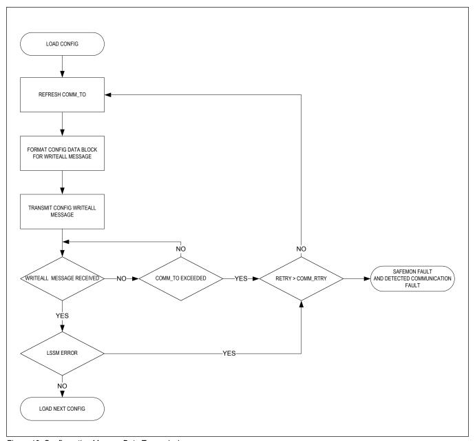
Figure 10. Configuration Memory Data Transmission
