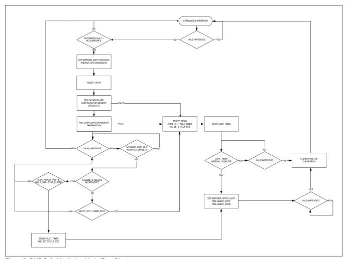
Figure 7. BMS Safe Monitoring Mode Flow Chart
