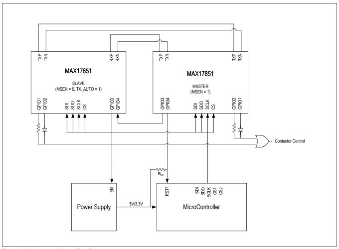
Figure 22. Hardware In Loop Test Setup
