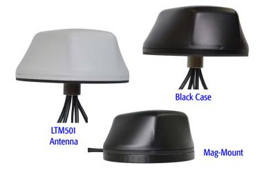
Mobile Mark's LTM501 Series Multiband Diversity/MIMO antenna contains five separate antennas, all in one compact antenna housing: two LTE 700 MHz & Cellular antennas, two dual-band WiFi antennas, and one GPS antenna.
