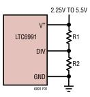
Figure 1. Simple Technique for Setting DIVCODE
