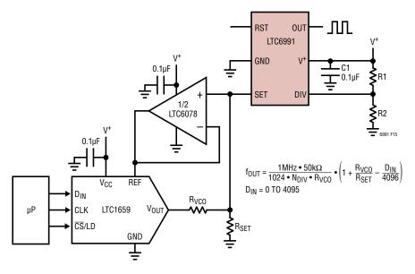
Figure 15. Digitally-Controlled Oscillator
