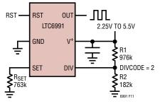
Figure 11. 1Hz Oscillator
