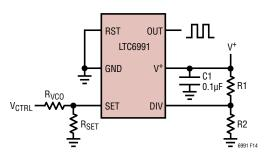
Figure 14. Voltage-Controlled Oscillator
