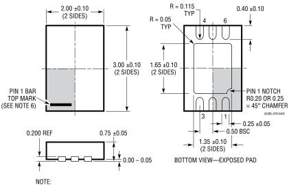
DCB Package 6-Lead Plastic DFN ( $2mm \times 3mm$ )
