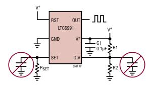
**RST (Pin 4/Pin 1):** Output Reset. The behavior of the RST pin is dependent on the polarity bit (POL). The POL bit is configured via the DIVCODE setting. When POL = 0, setting RST high forces OUT low and setting RST low allows the output to oscillate. When POL = 1, RST is active low. In that case, setting RST low forces OUT high and setting RST high allows the output to oscillate.
