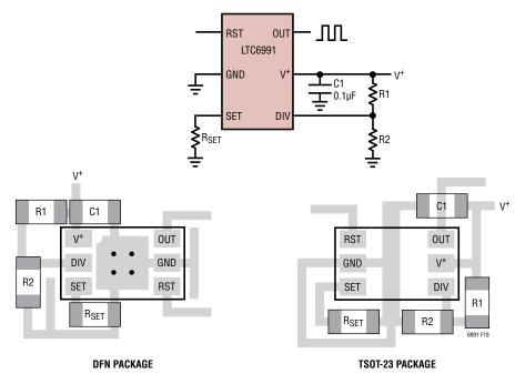
Figure 16. Supply Bypassing and PCB Layout
