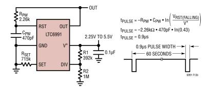
Figure 13b. Self-Resetting Circuit (DIVCODE = 11)
