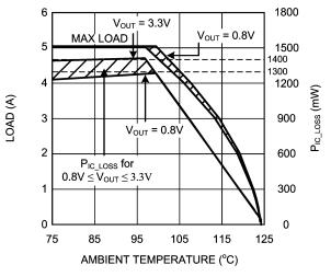
Figure 7. Current Derating vs. Ambient Temperature LMZ10505, V\_{IN} = 5.0V,  $\theta_{JA}$  = 20°C/W
