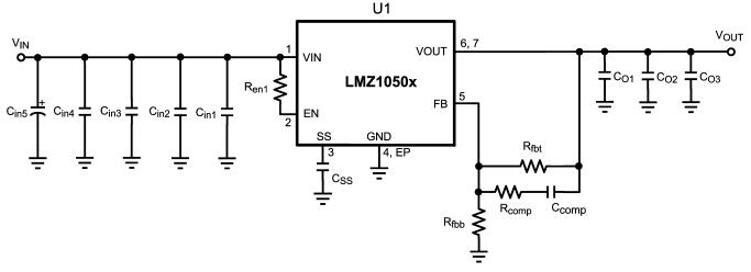
Figure 1. Component Schematic for Evaluation Board
