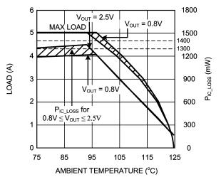
Figure 10. Current Derating vs. Ambient Temperature LMZ10505, V\_{IN} = 3.3V,  $\theta_{JA}$  = 20°C/W
