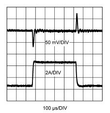
Figure 18. Load Transient Response  $V_{IN}$  = 3.3V,  $V_{OUT}$  = 2.5V LMZ10505,  $I_{OUT}$  = 500 mA to 4.5A, 20 MHz Bandwidth Limit
