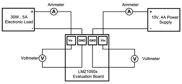
Figure 3. Efficiency Measurement Setup
