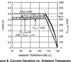
Figure 8. Current Derating vs. Ambient Temperature LMZ10503,  $V_{IN}$  = 3.3V,  $\theta_{JA}$  = 20°C/W
