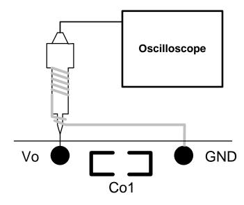
Figure 4. Output Voltage Ripple Measurement Setup
