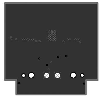
Figure 24. Internal Layer I (Ground)
