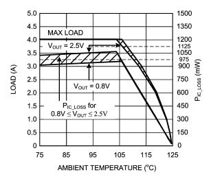
Figure 9. Current Derating vs. Ambient Temperature LMZ10504,  $V_{IN}$  = 3.3V,  $\theta_{JA}$  = 20°C/W
