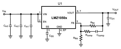
Figure 19. Component Schematic,  $V_{IN} = 5V$ ,  $V_{OUT} = 2.5V$ , Complies with EN55022 Class B Radiated Emissions
