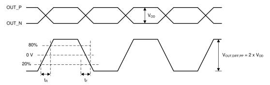
Figure 7-8. Differential Output Voltage and Rise/Fall Time
