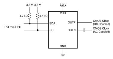
Figure 9-1. LMK61E07 Typical Application
