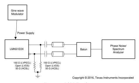
Figure 7-7. PSRR Test Setup
