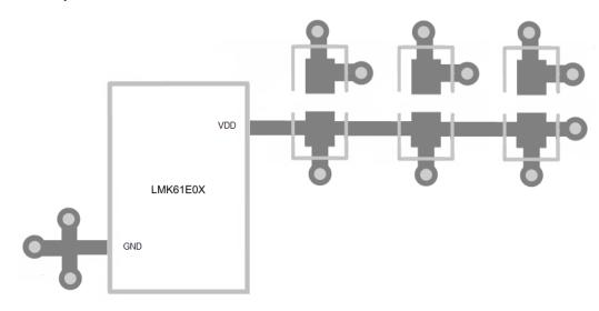
Figure 9-4. LMK61E07 Layout Recommendation for Power Supply and Ground
