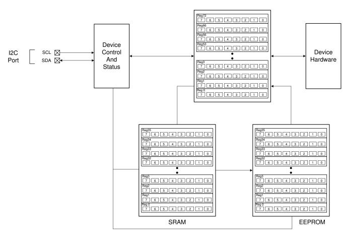
Figure 8-3. LMK61E07 Interface and Control Block
