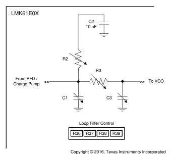
Figure 8-2. Loop Filter Structure of PLL
