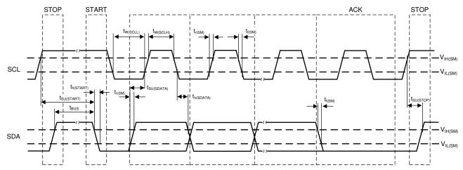
Figure 8-5. I<sup>2</sup>C Timing Diagram
