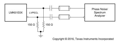
Figure 7-4. LVPECL Output AC Configuration During Device Test
