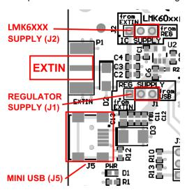
Figure 3. Power Terminals and Jumpers
