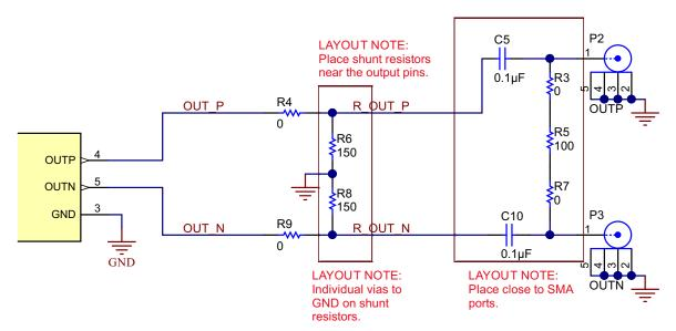
Figure 4. LMK6XXX Termination Schematic
