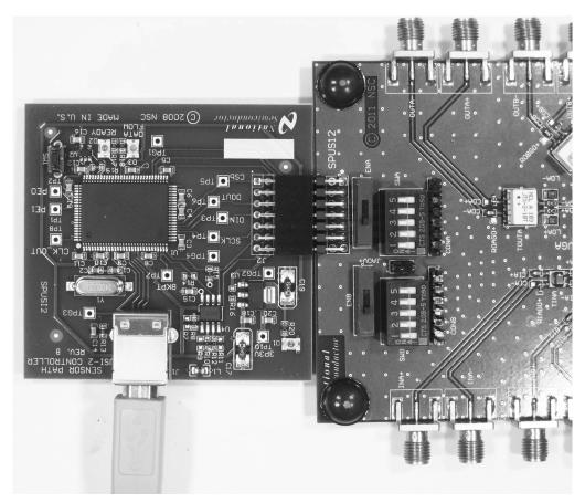
Figure 4. SPISU2 Card Connected to LMH6522EVAL Board
