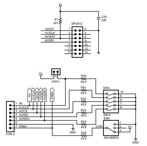
Figure 9. Logic Header Schematic
