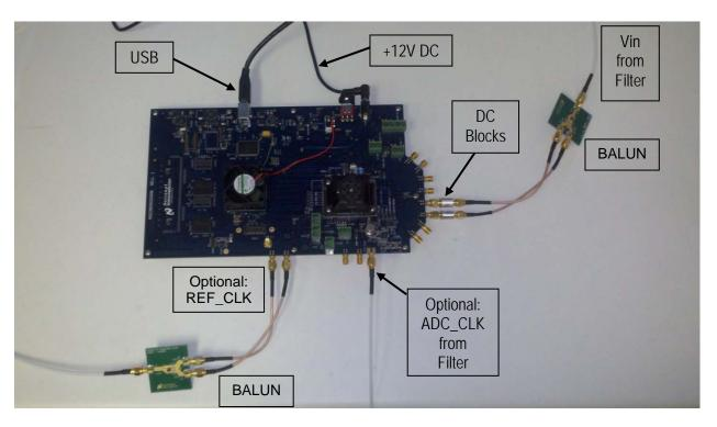
Figure 3: Recommended lab setup for on-board clock mode. A filter may not be necessary on the clock if the generator is very clean (beyond -80dBm SFDR).
