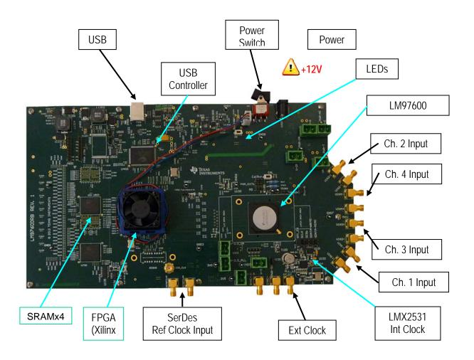
Figure 1: LM97600RB Board Layout
