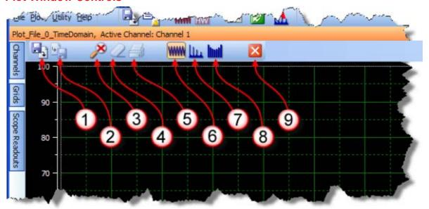
Figure 7: WaveVision 5 plot window controls
