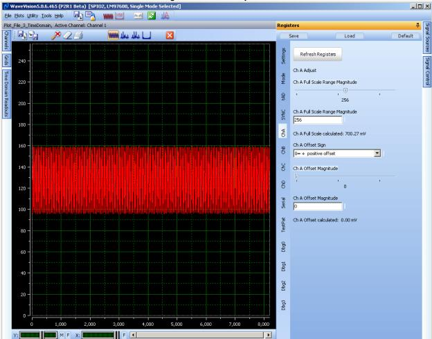
ChA: This tab controls the Full Scale Range and Offset adjustments for Channel A.
