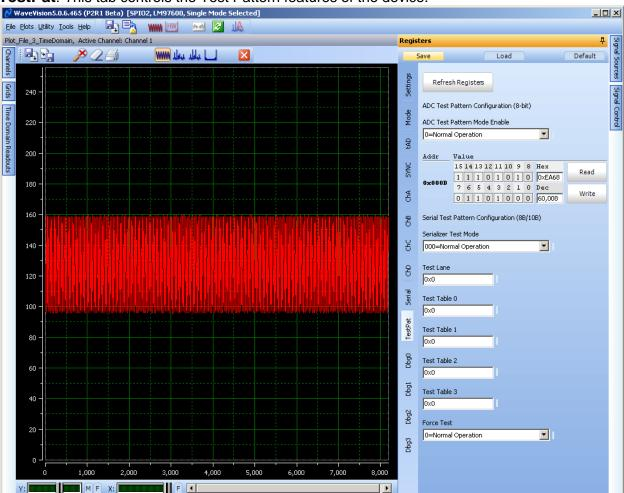
**TestPat**: This tab controls the Test Pattern features of the device.
