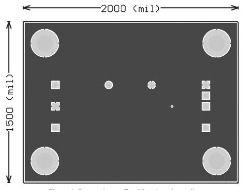
Figure 3. Bottom Layer, Top View (unmirrored)
