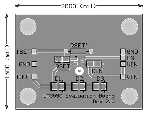
Figure 2. Top Layer, Top View
