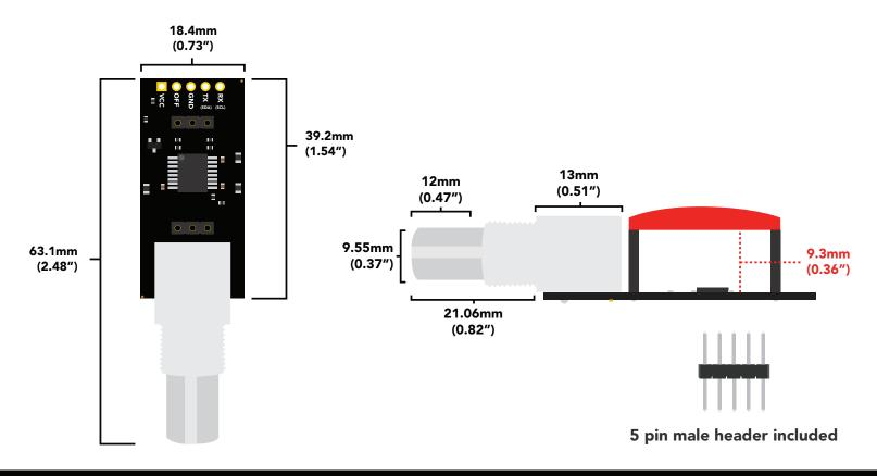
The Electrically Isolated EZO™ Carrier Board works with almost all EZO™ circuits, except the EZO™ Universal Flow Meter Totalizer.
