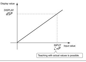
Instead of setting by inputting with the O Up Key and O Shift Key, current values can be input as scaling input values for teaching. This is useful for making settings while checking the operation status of the K3MA-F.
