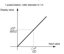
When displaying a flowrate (e.g., in  $\ell$ /min or  $\ell$ /h), make the scaling settings after confirming the I/O characteristics of the flowrate sensor. There are flowrate sensors that output analog signals. If this kind of flowrate sensor is used, consider using the K3MA-J.
