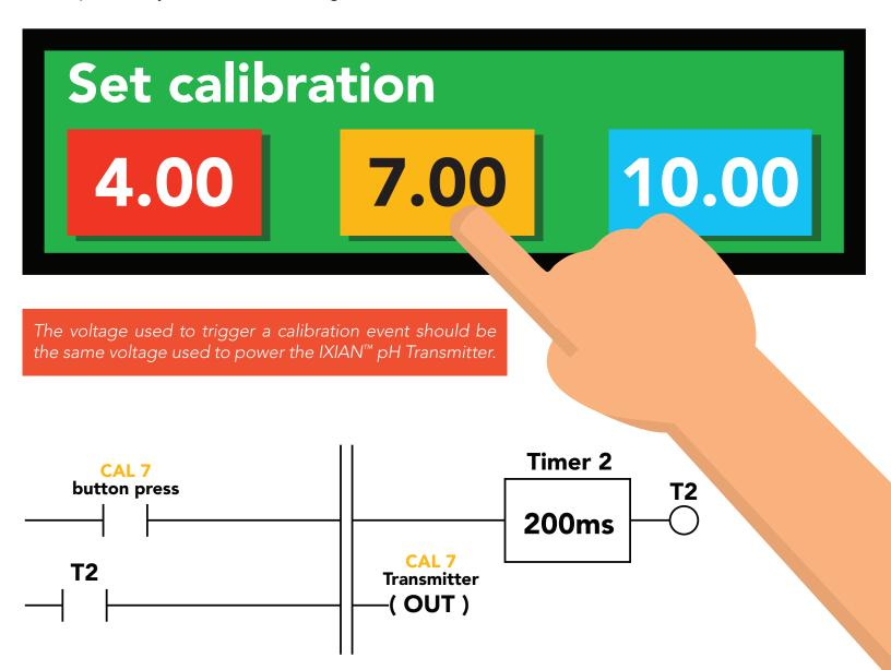
A calibration event will only trigger if the corresponding input pin has been held high for 200ms. Holding the line for more then 200ms will have no effect.
