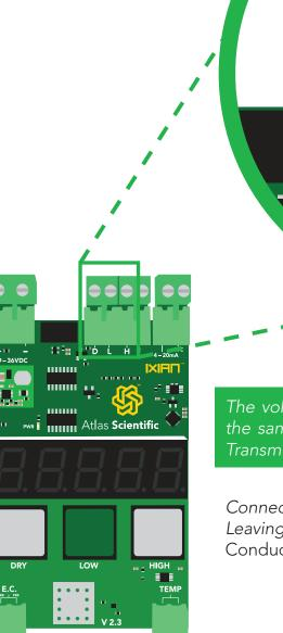
The voltage used to trigger a calibration event should be the same voltage used to power the IXIAN<sup>™</sup> Conductivity Transmitter.
