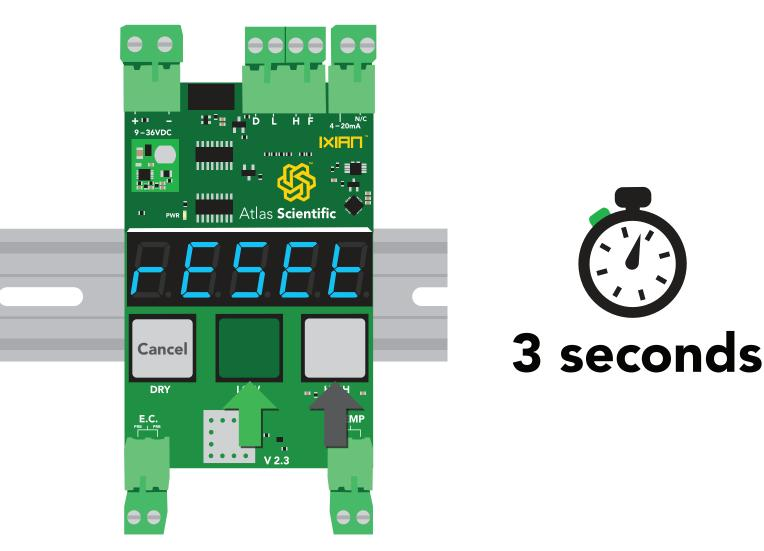
Press and hold the **LOW** and **HIGH** buttons again to confirm the factory reset. To cancel a factory reset, press the **DRY** button.
