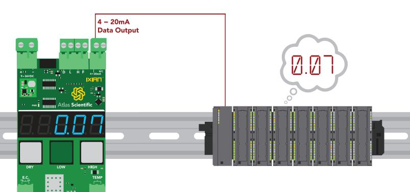
Connecting the 4 – 20mA data output to your PLC is **purely optional.** Leaving it disconnected will have no effect on the IXIAN<sup>™</sup> Conductivity Transmitter's operation.
