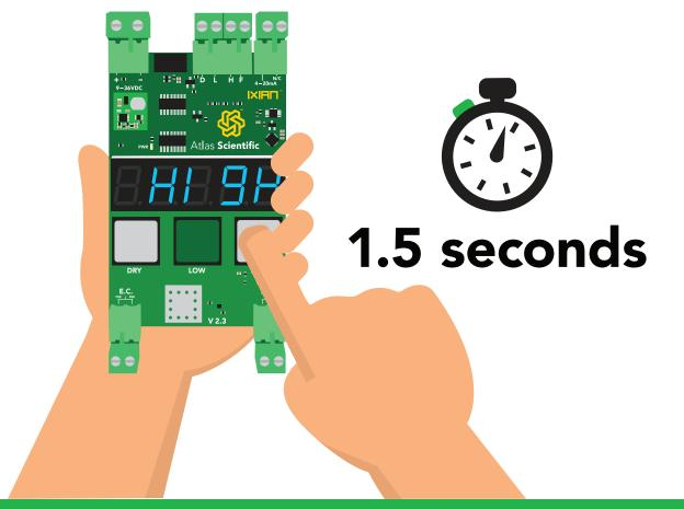
The conductivity readings will not change after low point calibration. The readings will change only when both high and low point calibration has been completed.
