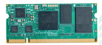
iWave's i.MX6UL based SODIMM CPU module integrates power efficient high performance ARM Cortex A7 CPU core operating up to 528MHz speed. The SOM is ultra-compact in size and integrated with on-board PMIC, Flash, DDR3 and dual Ethernet PHY. The SOM is ideally suitable for the cost & power optimized general embedded and industrial applications.
