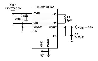
FIGURE 1. TYPICAL FIXED OUTPUT APPLICATION
