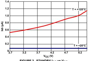
FIGURE 2. STANDBY I<sub>CC</sub> vs V<sub>CC</sub>
