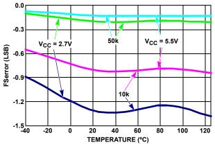
FIGURE 6. FSerror vs TEMPERATURE
