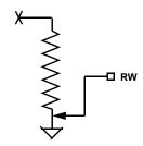
FIGURE 11. DCP CONNECTION IN SHUTDOWN MODE
