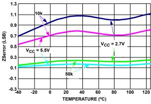
FIGURE 5. ZSerror vs TEMPERATURE
