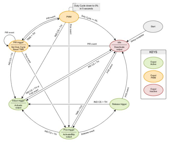
Figure 2.2: State diagram of the IQS680 output
