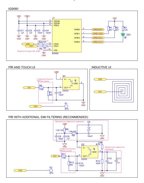
Figure 1.2 IQS680 reference schematic
