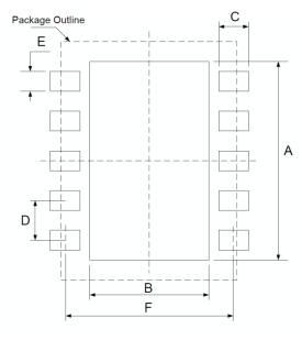
Figure 11.3: DFN-10 Landing dimensions
