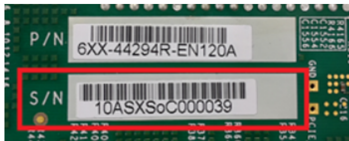
Figure 4-4: Board Serial Number Sticker
