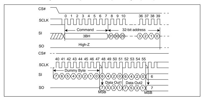
Figure 20. Dual Output Fast Read with 4-Byte Address Sequence Diagram (ADS=0 or ADS=1)
