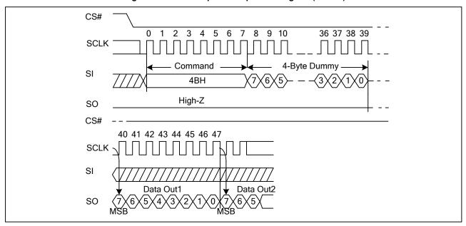
Figure 54. Read Unique ID Sequence Diagram (ADS=0)
