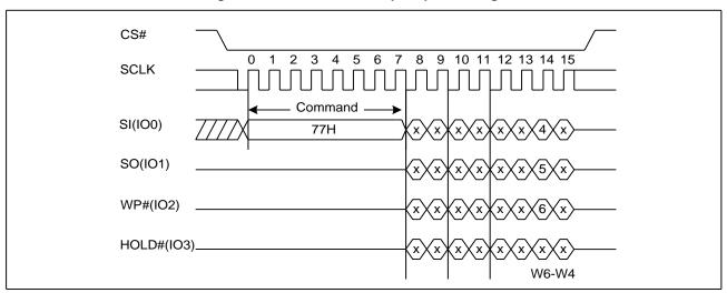
Figure 36. Set Burst with Wrap Sequence Diagram
