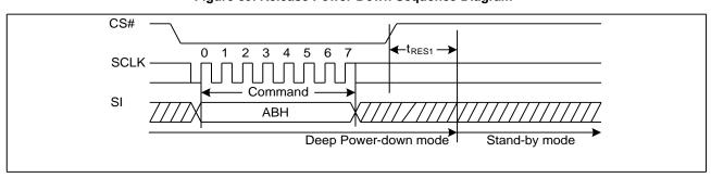
Figure 59. Release Power-Down Sequence Diagram
