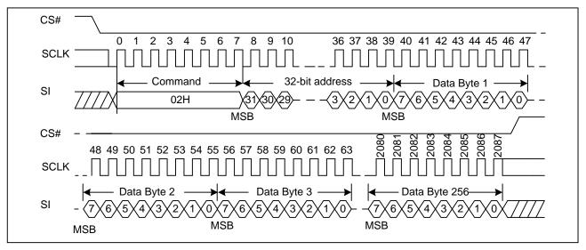
Figure 39. Page Program with 4-Byte Address Sequence Diagram (ADS=0 or ADS=1)
