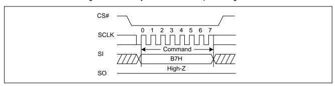
Figure 56. Enter 4-Byte Address Mode Sequence Diagram
