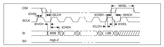
Figure 79. Output Timing
