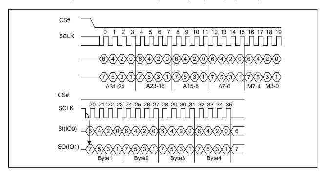
Figure 28. Dual I/O Fast Read with 4-Byte Address Sequence Diagram (M5-4≠ (1, 0), ADS=0 or ADS=1)
