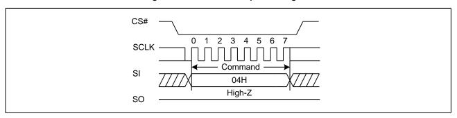
Figure 6. Write Disable Sequence Diagram
