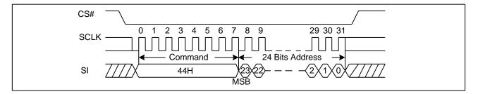
Figure 68. Erase Security Registers command Sequence Diagram (ADS=1)
