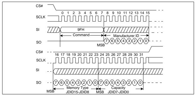
Figure 64. Read Identification ID Sequence Diagram
