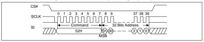
Figure 48. 32KB Block Erase with 4-Byte Address Sequence Diagram (ADS=0 or ADS=1)
