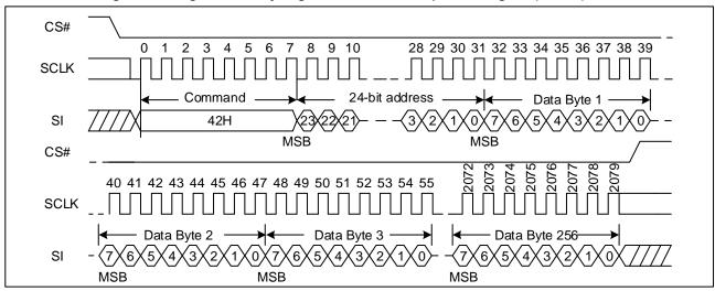
Figure 70.Program Security Registers command Sequence Diagram (ADS=1)
