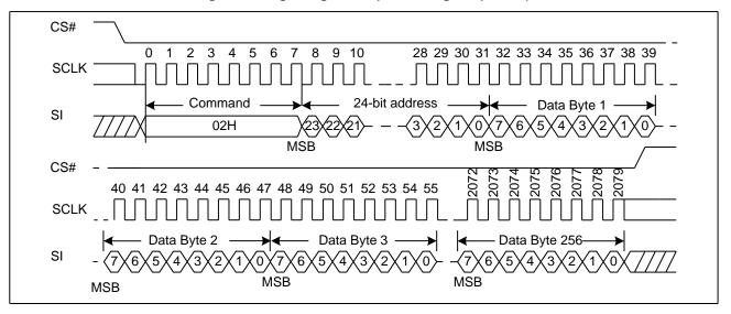
Figure 38. Page Program Sequence Diagram (ADS=1)
