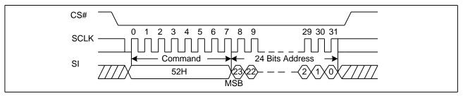
Figure 47.32KB Block Erase Sequence Diagram (ADS=1)
