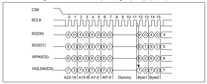
Figure 32. Quad I/O Fast Read Sequence Diagram (M5-4≠ (1, 0), ADS=1)
