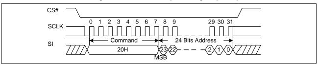
Figure 44. Sector Erase Sequence Diagram (ADS=1)
