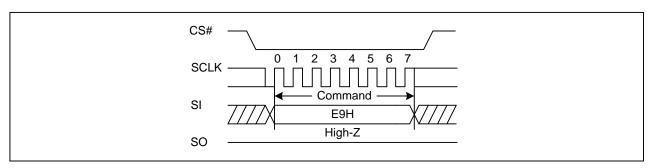
Figure 57.Exit 4-Byte Address Mode Sequence Diagram
