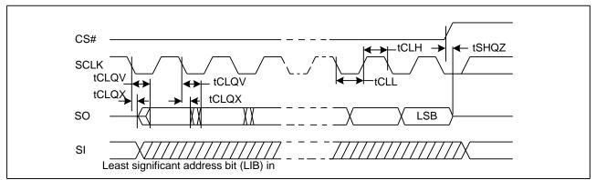
Figure 80. Resume to Suspend Timing
