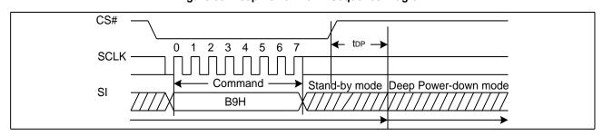
Figure 53. Deep Power-Down Sequence Diagram
