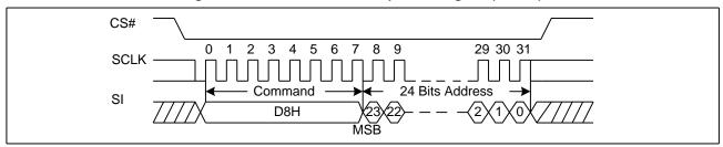
Figure 50.64KB Block Erase Sequence Diagram (ADS=1)
