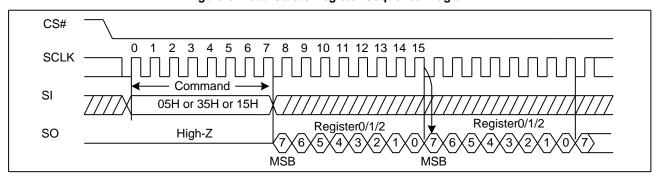
Figure 8. Read Status Register Sequence Diagram
