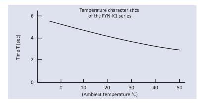
Damper characteristics vary according to the ambient temperature. In general, the damper characteristics become weaker as the temperature increases, and become stronger as the temperature decreases. This is because the viscosity of the oil inside the damper varies according to the temperature. When the temperature returns to normal, the damper characteristics will return to normal as well. The changes in the time it takes for the lid to close are shown in the graph to the left.
