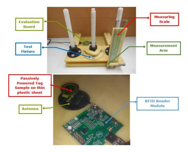
The test sample is placed on a thin sheet of plastic connected to the movable part of the fixture. Then the distance is carefully adjusted until the reader can no longer read the sample, thus the maximum interrogation distance is displayed in the ruler.
