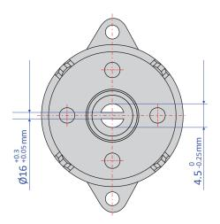
The FDT-70B-903 has a slotted groove which is excellent for usage with spiral springs
