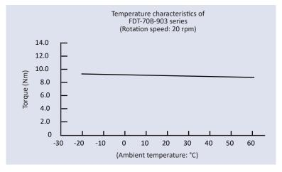
rated torque in this document) varies according to the ambient temperature. As the temperature increases, the torque decreases, and as the temperature decreases, the torque increases. This is because the viscosity of the silicone oil inside the damper varies according to the temperature. The graph to the left illustrates the temperature characteristics.
