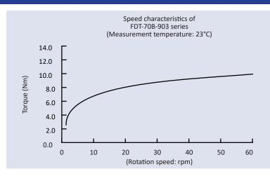
Speed characteristics: A disk damper's torque varies according to the rotation speed. In general, as shown in the graph to the left, the torque increases as the rotation speed increases, and the torque decreases as the rotation speed decreases. Torque at 20 rpm is shown in this document. In a closing lid, the rotation speed is slow when the lid begins to close, resulting in the generation of torque that is smaller than the rated torque.
