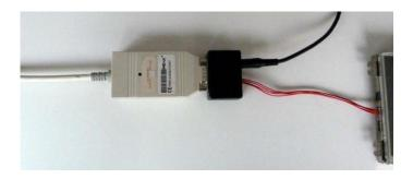
For all other versions of StarterKit not equipped with the communication interface, all you have to do is wire a bundle bringing your + 12Vdc / 1A power supply and your CAN interface according to the J702 connector specification:
