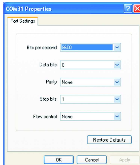
Figure 36. 9600 bps With No Flow Control
