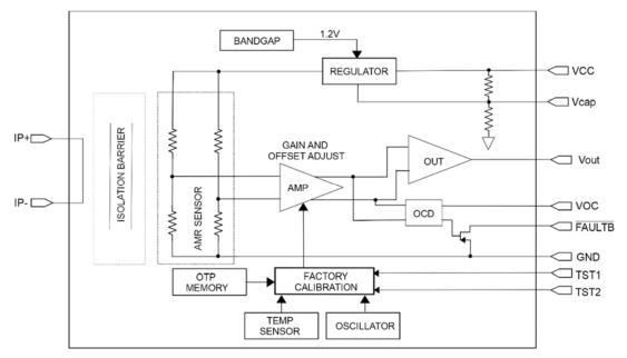
Figure 2 - Block diagram for ratiometric gain products
