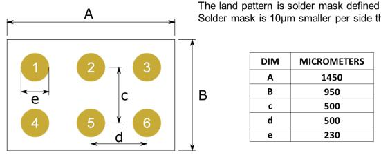
Solder mask is 10µm smaller per side than bump
