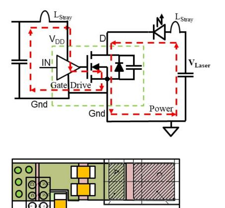
Cathode to drain connection on second conductor layer.
