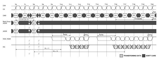
NOTE 1. BC = 4, RL = 11 (CL = 11, AL = 0), Read Preamble = 2t<sub>CK</sub>. WL = 10 (CWL = 9+1<sup>15</sup>, AL = 0), Write Preamble = 2t<sub>CK</sub>
