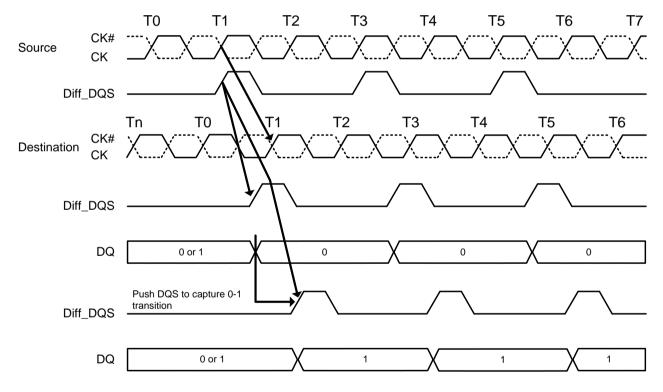
Figure 12. Write Leveling Concept
