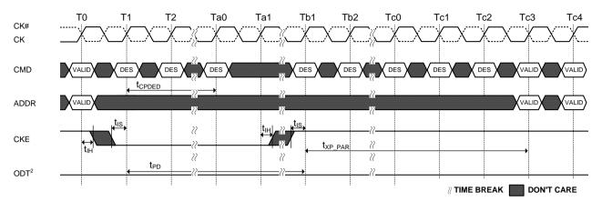
NOTE 1 VALID command at T0 is ACT, DES or Precharge with still one bank remaining open after completion of the precharge command. NOTE 2 ODT pin driven to a valid state, MR5[A5 = 0] (default setting) is shown NOTE 3 CA Parity = Enable
