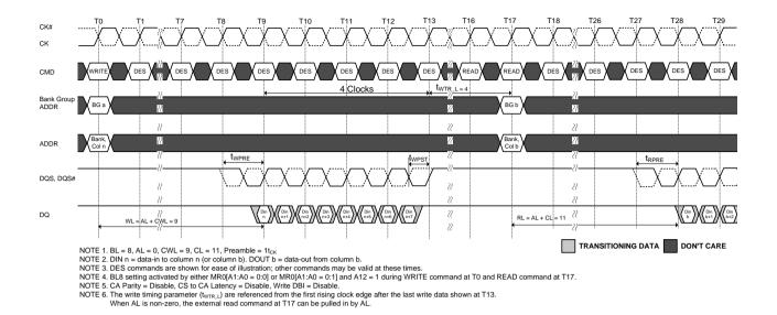
Figure 135. WRITE (BL8) to READ (BL8) with 1t<sub>CK</sub> Preamble in Same Bank Group
