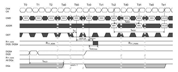
Figure 14. Write Leveling Exit
