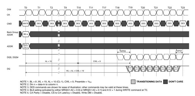
Figure 126. WRITE Burst Operation WL = 19 (AL = 10, CWL = 9, BL8)
