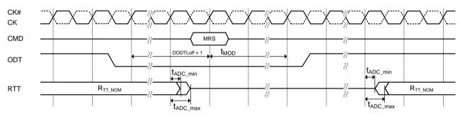
NOTE 1. This timing diagram shows C/A Parity Latency mode is "Disable" case.
