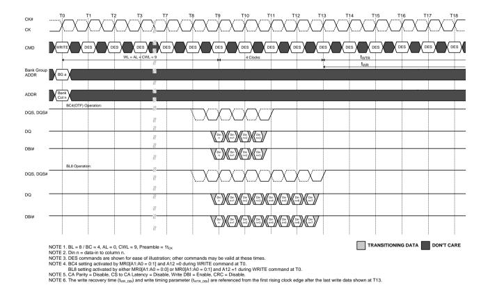
Figure 146. WRITE (BL8/BC4) OTF with 1t<sub>CK</sub> Preamble and DBI
