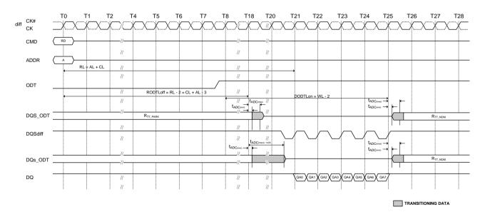
Figure 167. Example: CL=11, PL=0; AL=CL-1=10; RL=AL+PL+CL=21; CWL=9; DODTLon=AL+CWL-2=17; DODTLoff=AL+CWL-2=17; 2tCK preamble)
