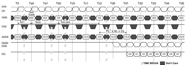
NOTE 1. Multi-Purpose Registers Read/Write Enable (MR3 A2 = 1)
