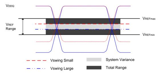
Figure 44. V<sub>REFDQ</sub> Operating Range (V<sub>REFmin</sub>, V<sub>REFmax</sub>)
