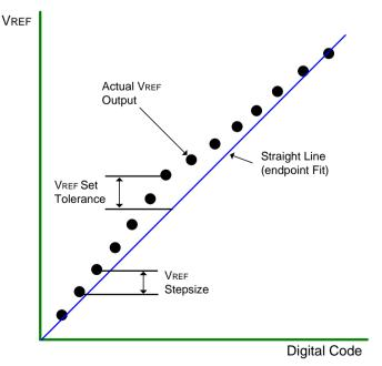
Figure 45. Example of V<sub>REF</sub> set tolerance (max case only shown) and stepsize
