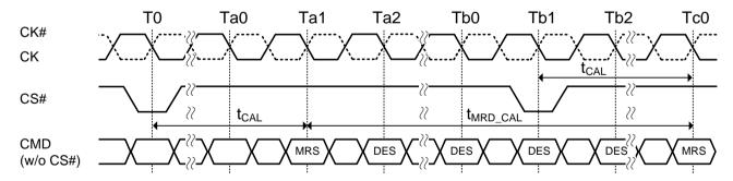
NOTE1: MRS at Ta1 may or may not modify CAL,  $t_{MRD\_CAL}$  is computed based on new  $t_{CAL}$  setting. NOTE2:  $t_{MRD\_CAL} = t_{MOD} + t_{CAL}$
