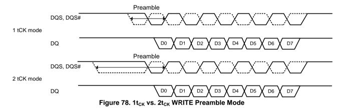
The timing diagrams contained in  $t_{\text{CCD}}$ =4 (AL=PL=0),  $t_{\text{CCD}}$ =5 and  $t_{\text{CCD}}$ =6 (AL=PL=0) illustrate 1 and 2  $t_{\text{CK}}$  preamble scenarios for consecutive write commands with  $t_{\text{CCD}}$  timing of 4, 5 and 6 nCK, respectively. Setting t<sub>CCD</sub> to 5nCK is not allowed in 2 t<sub>CK</sub> preamble mode.
