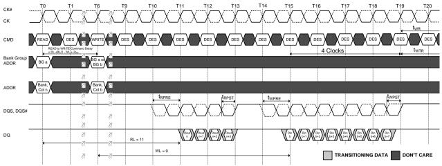
NOTE 1. BC = 4, RL = 11(CL = 11, AL = 0), Read Preamble = 1t<sub>CK</sub>, WL=9(CWL=9,AL=0), Write Preamble = 1t<sub>CK</sub>
