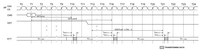
Figure 169. Dynamic ODT overlapped with Rtt\_NOM (CL=14, CWL=11, BL=8, AL=0, CRC Disabled)
