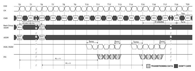
NOTE 1. BC = 4, RL = 11 (CL = 11, AL = 0), Read Preamble = 1t<sub>CK</sub>, WL = 9 (CWL = 9, AL = 0), Write Preamble = 1t<sub>CK</sub> NOTE 2. Dout n = data-out from column n, DIN b = data-in to column b.
