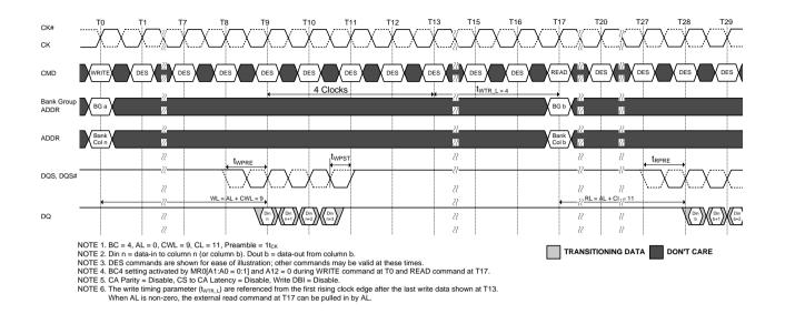
Figure 137. WRITE (BC4)OTF to READ (BC4)OTF with 1t<sub>CK</sub> Preamble in Same Bank Group
