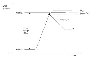
Figure 50. VREF full step from VREFmin to VREFmax case
