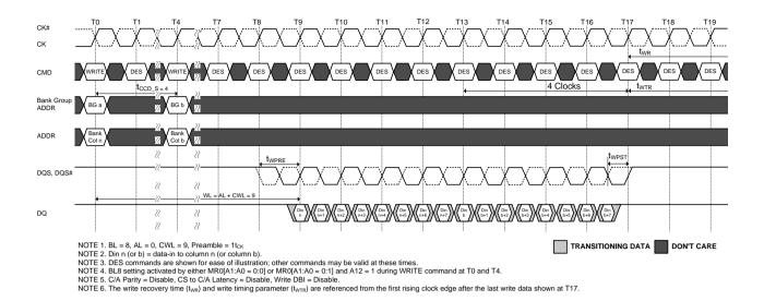
Figure 127. Consecutive WRITE (BL8) with 1t<sub>CK</sub> Preamble in Different Bank Group
