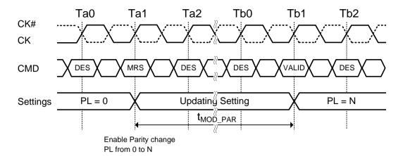
NOTE 1. tMOD\_PAR = tMOD + N; where N is the programmed parity latency with the MRS command entering CA parity mode.
