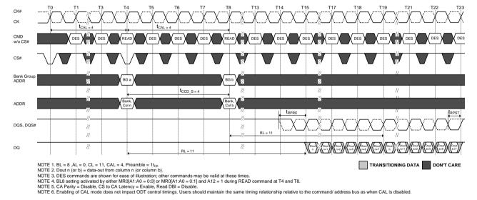
Figure 122. Consecutive READ (BL8) with CAL(4) and 1t<sub>CK</sub> Preamble in Different Bank Group
