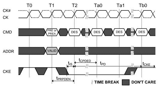
Figure 35. Precharge/Precharge all Command Power-Down Entry
