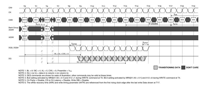
Figure 140. WRITE (BL8) to WRITE (BC4) OTF with 1t<sub>CK</sub> Preamble in Different Bank Group
