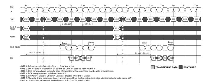
Figure 138. WRITE (BC4)Fixed to READ (BC4)Fixed with 1t<sub>CK</sub> Preamble in Different Bank Group
