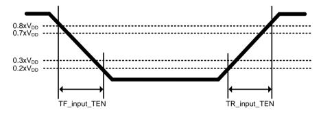
Figure 155. TEN Input Slew Rate Definition
