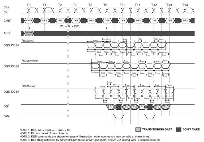
Figure 123. Write Timing Definition and Parameters with 1t<sub>CK</sub> Preamble
