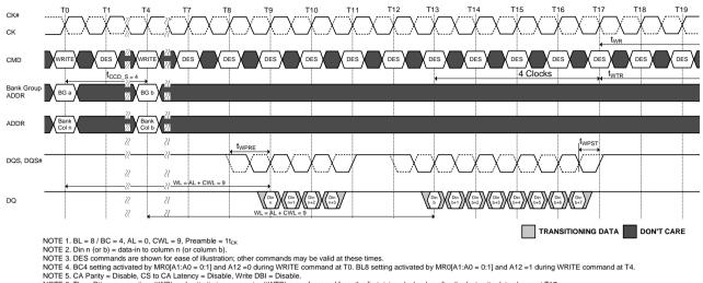
NOTE 6. The wRife recovery time (tWR) and write timing parameter (tWTR) are referenced from the first rising clock edge after the last write data shown at T17
