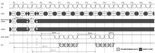
NOTE 1. BL = 8, AL = 0, CL = 11, Preamble =  $2t_{\rm CK}$ NOTE 2. Dout n (or b) = data-out from column n (or column b). NOTE 3. DES commands are shown for ease of illustration; other commands may be valid at these times. NOTE 4. BC4 setting activated by either MRO[AT:A0 = 1:0] or MRO[AT:A0 = 0:1] and A12 = 0 during READ command at T0 and T4. NOTE 5. CA Parity = Disable, CS to CA Latency = Disable, Read DBI = Disable
