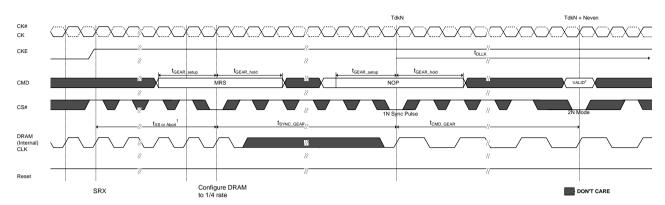
NOTE 1. CKE High Assert to Gear Down Enable Time (tXS, tXS\_Abort) depend on MR setting. A correspondence of tXS/tXS\_Abort and MR Setting is as follows.
