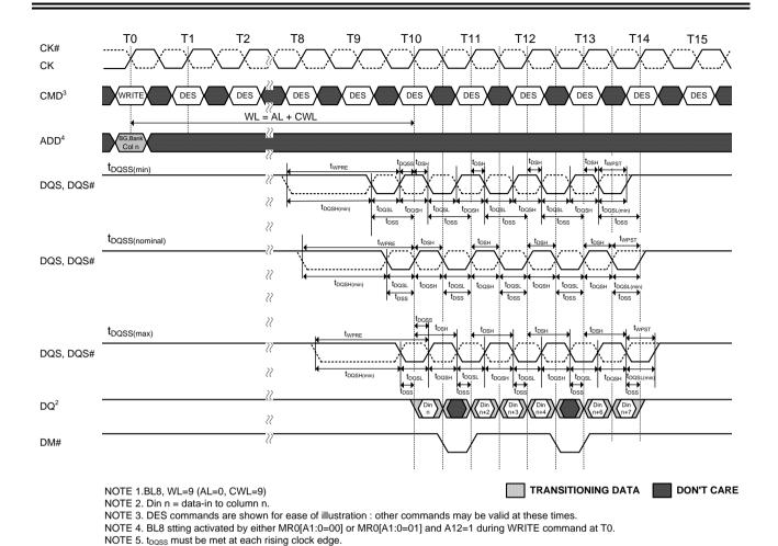
Figure 124. Write Timing Definition and Parameters with 2t<sub>CK</sub> Preamble
