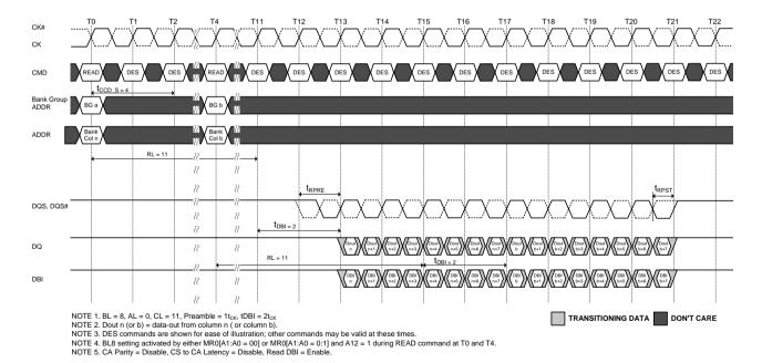
Figure 116. Consecutive READ (BL8) with 1t<sub>CK</sub> Preamble and DBI in Different Bank Group
