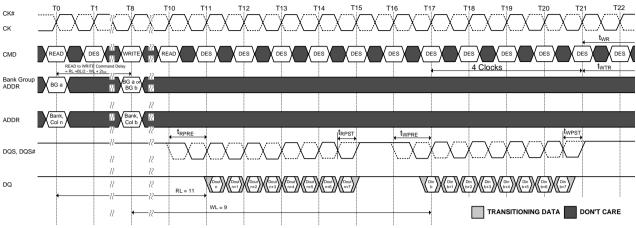
NOTE 1. BL = 8, RL = 11 (CL = 11, AL = 0), Read Preamble = 1t<sub>CK</sub>, WL = 9 (CWL = 9, AL = 0), Write Preamble = 1t<sub>CK</sub>
