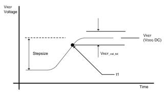
Figure 48. VREF step single stepsize increment case
