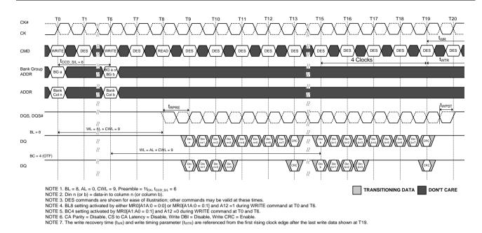
Figure 151. Nonconsecutive WRITE (BL8/BC4) OTF with 1t<sub>CK</sub> Preamble and Write CRC in Same or Different Bank Group
