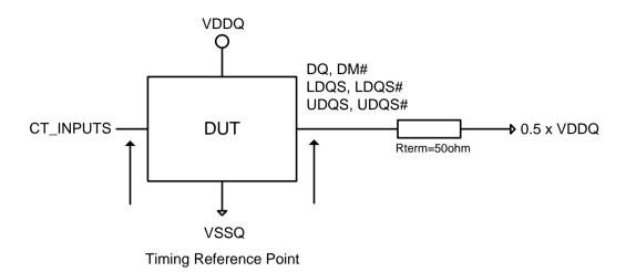
Figure 182. Connectivity Test Mode Timing Reference Load
