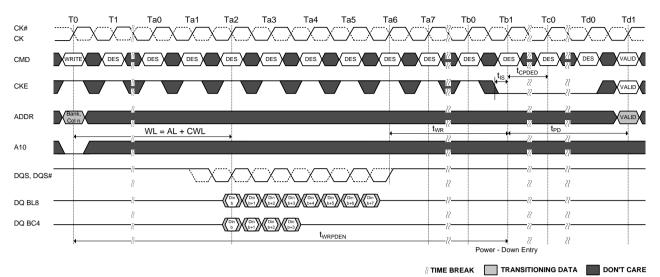
Figure 31. Power-Down Entry After Write
