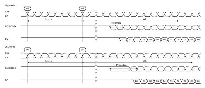
Figure 79. t<sub>CCD</sub>=4 (AL=PL=0)
