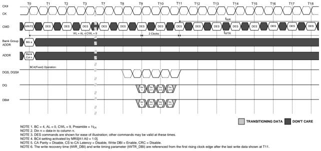
Figure 147. WRITE (BC4) Fixed with 1t<sub>CK</sub> Preamble and DBI
