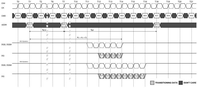
NOTE 1. BL = 8, RL = 11(CL = 11 , AL = 0 ), Preamble = 1t<sub>CK</sub>, t<sub>RTP</sub> = 6, t<sub>RP</sub> = 11
