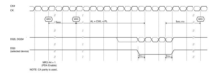
Figure 54. PDA using Burst Chop 4
