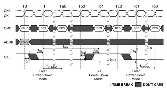
Figure 37. Power-Down Entry/Exit Clarification
