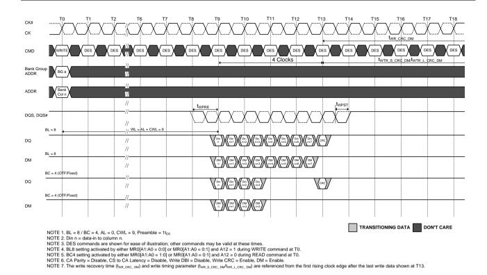
Figure 153. WRITE (BL8/BC4) OTF/Fixed with 1t<sub>CK</sub> Preamble and Write CRC and DM in Same or Different Bank Group
