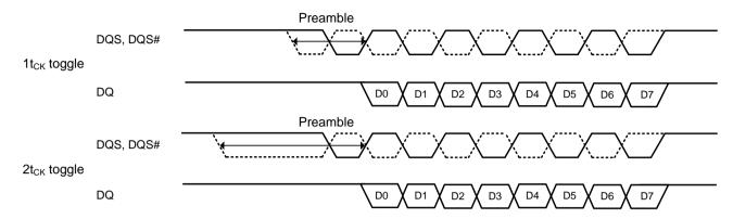
Figure 82. 1t<sub>CK</sub> vs. 2t<sub>CK</sub> READ Preamble Mode
