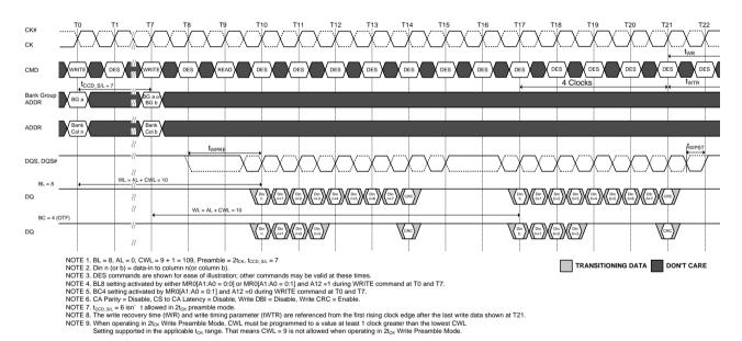
Figure 152. Nonconsecutive WRITE (BL8/BC4) OTF with 2t<sub>CK</sub> Preamble and Write CRC in Same or Different Bank Group
