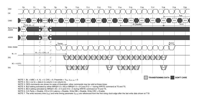
Figure 149. Consecutive WRITE (BL8/BC4) OTF with 1t<sub>CK</sub> Preamble and Write CRC in Same or Different Bank Group
