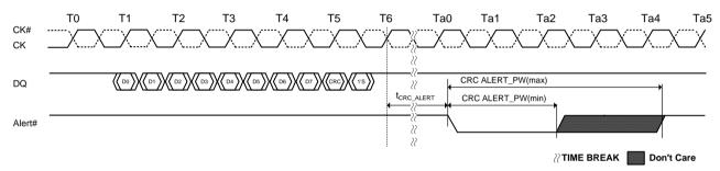
NOTE 1. CRC ALERT\_PW IS Specified from the point Where the DRAM starts to drive the signal low to the point where the DRAM driver releases and the controller starts to pull the signal up.
