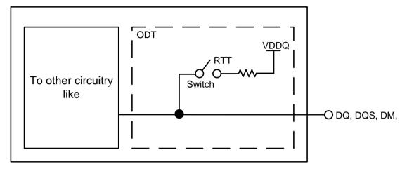
Figure 162. Functional Representation of ODT
