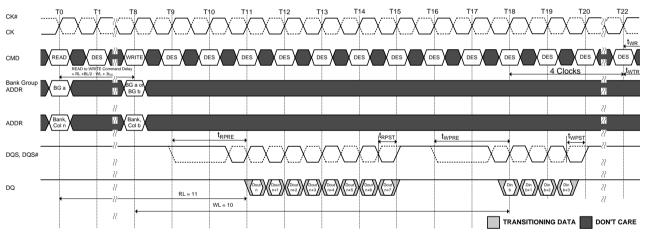
NOTE 1. BL = 8, RL = 11 (CL = 11, AL = 0), Read Preamble = 2t<sub>CK</sub>. WL = 10 (CWL = 9+1\*5, AL = 0), Write Preamble = 2t<sub>CK</sub>
