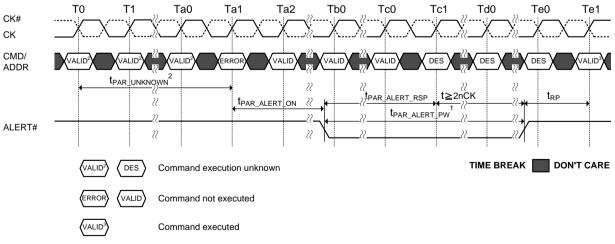
NOTE 1. DRAM is emptying queues, Precharge All and parity check re-enable finished by tPAR\_ALERT\_PW.
