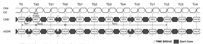
NOTE 1. Multi-Purpose Registers Read/Write Enable (MR3 A2 = 1) Redirect all subsequent read and writes to MPR locations
