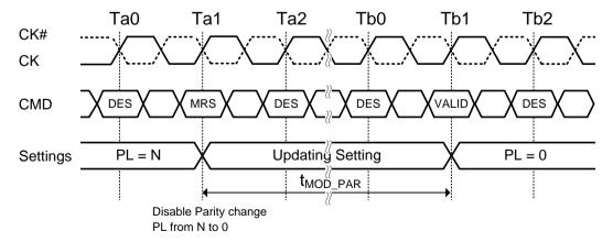
NOTE 1. tMOD\_PAR = tMOD + N; where N is the programmed parity latency prior to the MRS command exiting CA parity mode.
