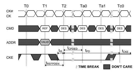
Figure 33. Refresh Command Power-Down Entry
