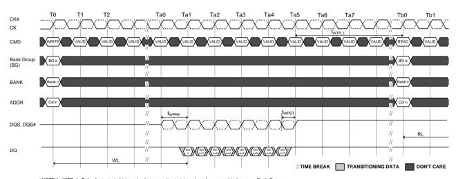
NOTE 1. tWTR\_L: Delay from start of internal write transaction to internal read command to the same Bank Group.
