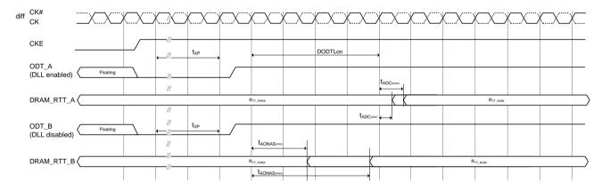
Figure 172. ODT timing for power down exit with ODT buffer disable mode
