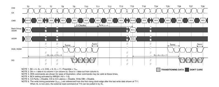
Figure 139. WRITE (BC4)Fixed to READ (BC4)Fixed with 1t<sub>CK</sub> Preamble in Same Bank Group
