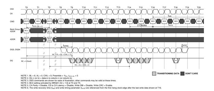
Figure 150. Consecutive WRITE (BC4) Fixed with 1t<sub>CK</sub> Preamble and Write CRC in Same or Different Bank Group
