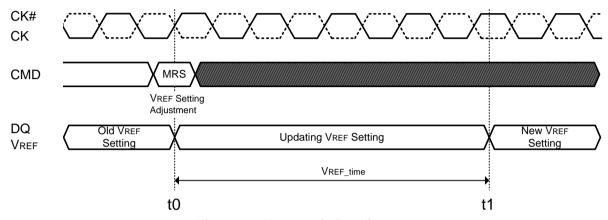
Figure 46. V<sub>REF time</sub> timing diagram
