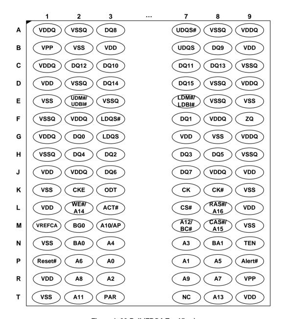
Figure 1. 96-Ball (FBGA Top View)
