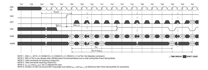
Figure 26. Self Refresh Exit with No Operation command
