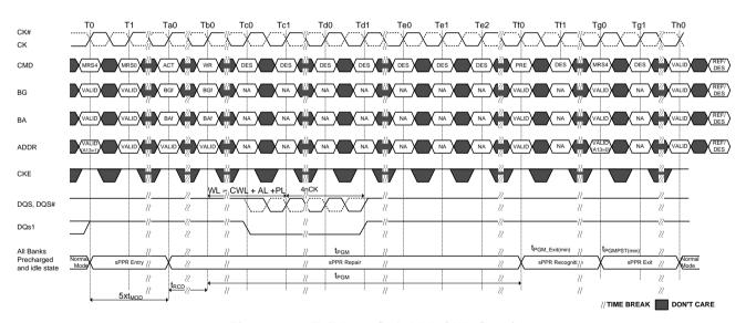
Figure 161. Fail Row Soft PPR (WR Case)
