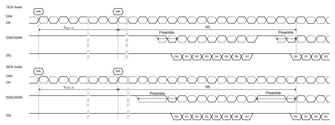
Figure 81. t<sub>CCD</sub>=6 (AL=PL=0)
