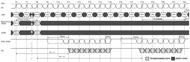
NOTE 1. BL = 8, RL = 11 (CL = 11, AL = 0), Read Preamble = 2t<sub>CK</sub>, WL = 10 (CWL = 9+1\*5, AL = 0), Write Preamble = 2t<sub>CK</sub>
