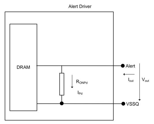
Figure 180. ALERT# output Drive Characteristic
