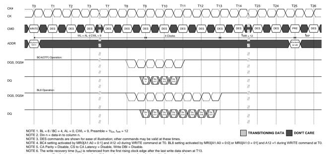
t<sub>WR</sub> specifies the last burst write cycle until the precharge command can be issued to the same bank.
