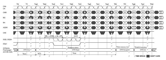
Figure 160. Hard Fail Row Repair (WR Case)
