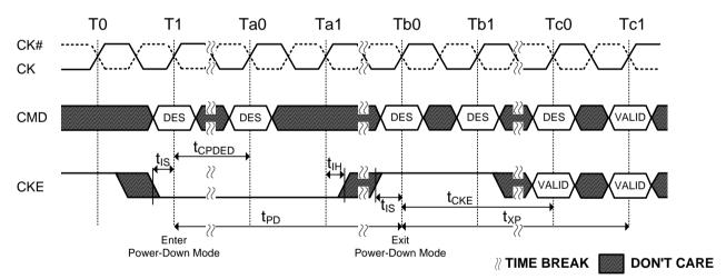
Figure 32. Precharge Power-Down Entry and Exit
