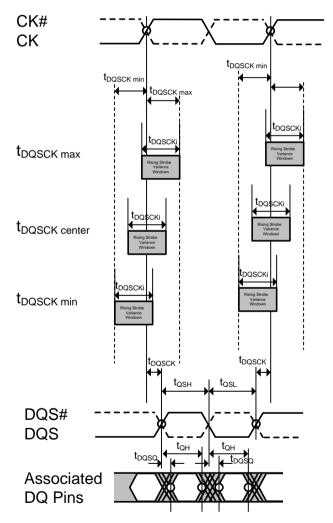
Figure 86. READ Timing Definition
