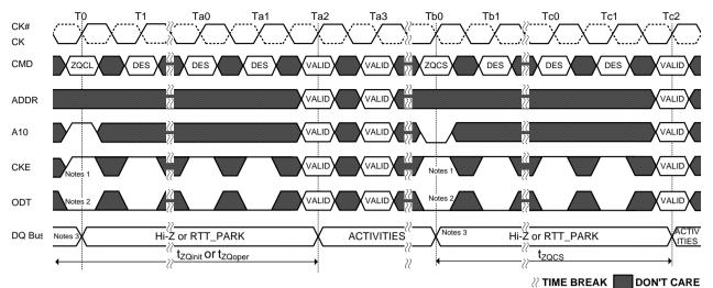
NOTE 1. CKE must be continuously registered high during the calibration procedure.
