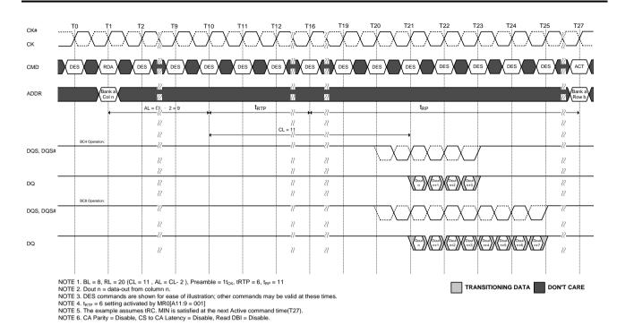
Figure 115. READ with Auto Precharge, Additive Latency and 1t<sub>CK</sub> Preamble
