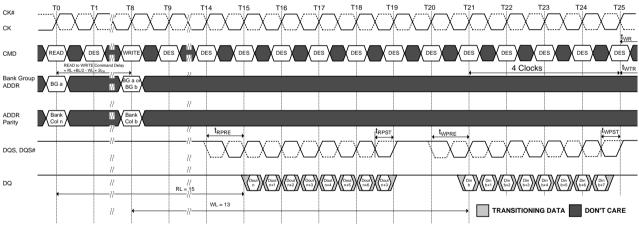
NOTE 1. BC = 4, RL = 11(CL = 11 , AL = 0 ), Read Preamble = 1t<sub>CK</sub>, WL=9(CWL=9,AL=0), Write Preamble = 1t<sub>CK</sub>
