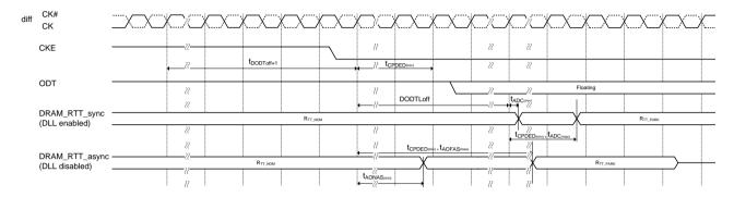
Figure 171. ODT timing for power down entry with ODT buffer disable mode
