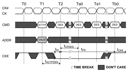
Figure 34. Activate Command Power-Down Entry
