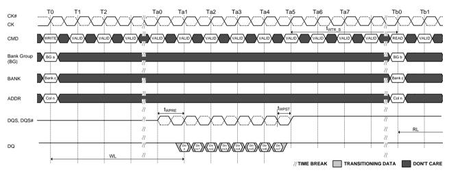
NOTE 1. tWTR\_S: Delay from start of internal write transaction to internal read command to a different Bank Group.
