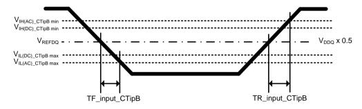
Figure 157. Input B Slew Rate Definition
