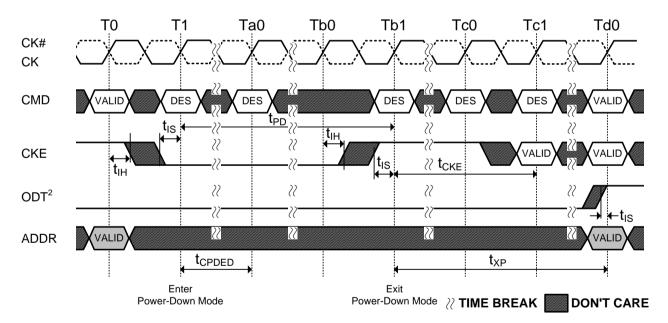
NOTE 1. Valid command at T0 is ACT, DES or Precharge with still one bank remaining open after completion of the precharge command.
