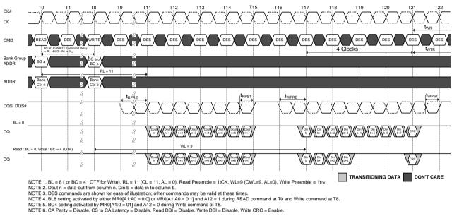
Figure 119. READ (BL8) to WRITE (BL8 or BC4: OTF) with 1t<sub>CK</sub> Preamble and Write CRC in Same or **Different Bank Group**
