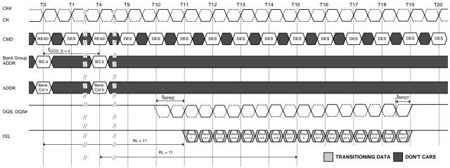
NOTE 1. BL = 8, AL = 0, CL = 11, Preamble = 1tCK NOTE 2. Dout n (or b) = data-out from column n (or column b).
