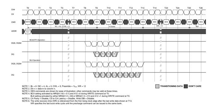
Figure 144. WRITE (BL8/BC4) OTF with Auto PRECHARGE Operation and 1t<sub>CK</sub> Preamble
