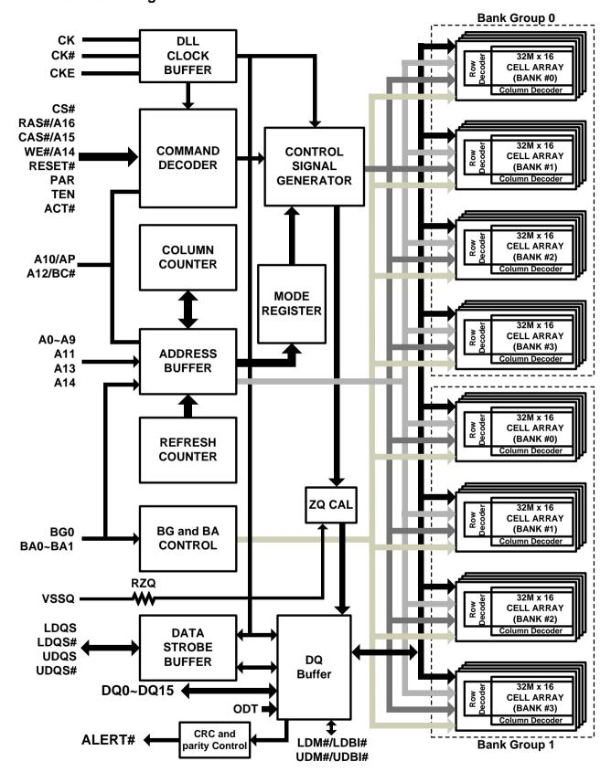
Figure 2. Block Diagram
