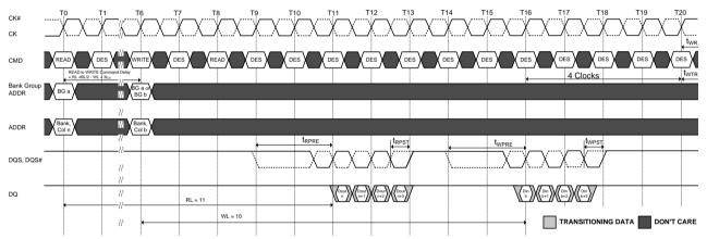
NOTE 1. BC = 4, RL = 11 (CL = 11, AL = 0), Read Preamble =  $2t_{CK}$ , WL = 10 (CWL = 9+1\*5, AL = 0), Write Preamble =  $2t_{CK}$  NOTE 2. Dout n = data-out from column n, DIN b = data-in to column b.
