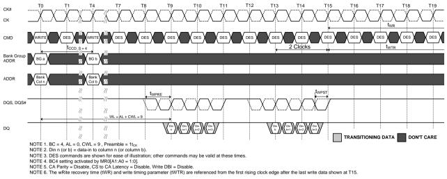
Figure 133. WRITE (BC4) Fixed to WRITE (BC4) Fixed with 1t<sub>CK</sub> Preamble in Different Bank Group
