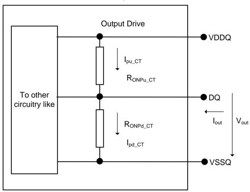
Figure 181. Output Driver Characteristic of Connectivity Test
