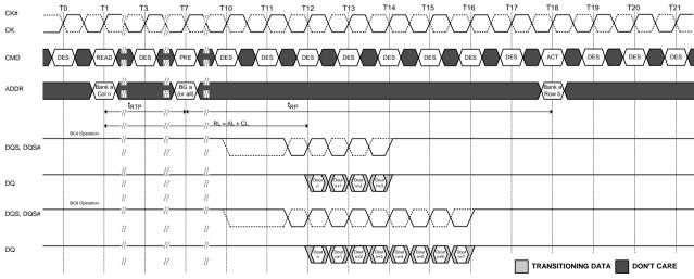
NOTE 1. BL = 8, RL = 11(CL = 11, AL = 0), Preamble =  $2t_{CK}$ ,  $t_{RTP}$  = 6,  $t_{RP}$  = 11
