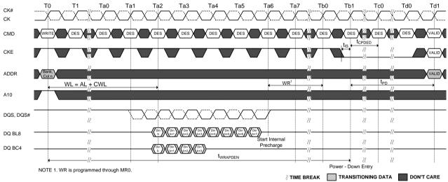
Figure 30. Power-Down Entry After Write with Auto Precharge
