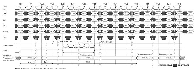
NOTE 1. Allow REF(1X) from PL+WL+BL/2+t<sub>WR</sub>+t<sub>RP</sub> after WR
