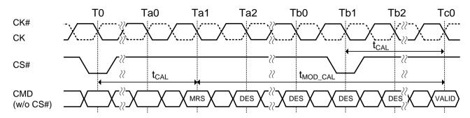
NOTE1: MRS at Ta1 may or may not modify CAL,  $t_{MOD\_CAL}$  is computed based on new  $t_{CAL}$  setting. NOTE2:  $t_{MOD\_CAL} = t_{MOD} + t_{CAL}$
