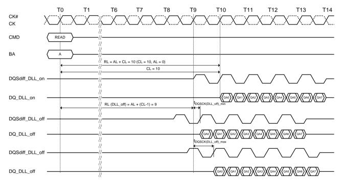
Figure 11. Read operation at DLL-off mode
