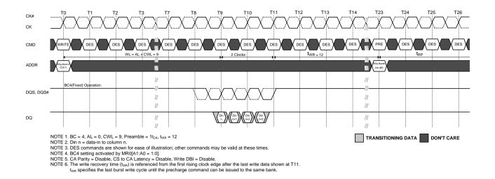
Figure 143. WRITE (BC4) Fixed to PRECHARGE Operation with 1t<sub>CK</sub> Preamble
