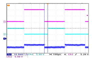
FIGURE 8. TRANSIENT LOAD RESPONSE
