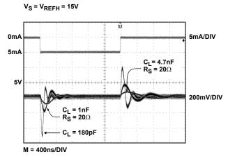
FIGURE 3. TRANSIENT LOAD REGULATION (SOURCING)
