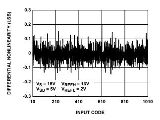
FIGURE 1. DIFFERENTIAL NONLINEARITY vs CODE
