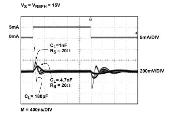
FIGURE 4. TRANSIENT LOAD REGULATION (SINKING)
