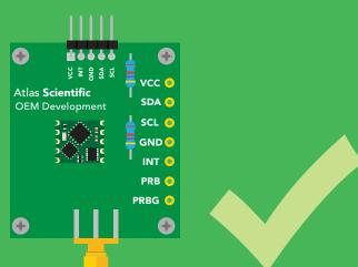
Do not solder wires to this device.
