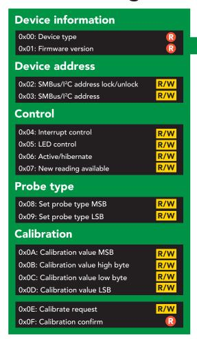
The default device address is **0x64** This address can be changed.
