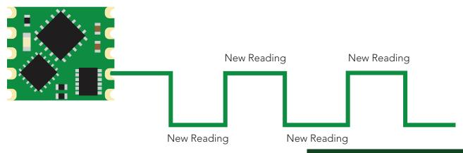
The pin will automatically invert its state each time a new reading is available. This setting has been specifically designed for a master device that can use an interrupt on change function.
