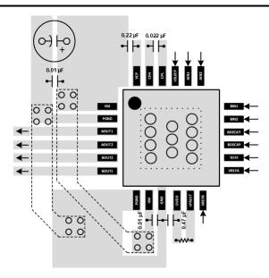
Figure 10-2. QFN Layout Recommendation
