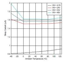
Figure 6-2. Sleep Current over Temperature
