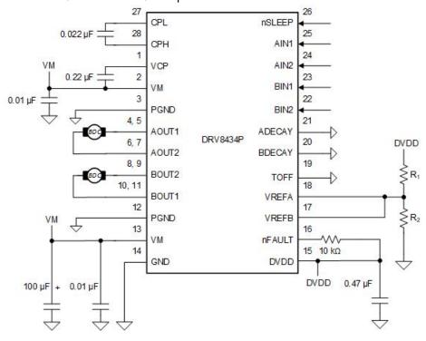
Figure 8-1. Typical Application Schematic
