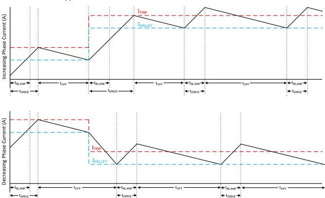
Figure 7-8. Smart tune Ripple Control Decay Mode
