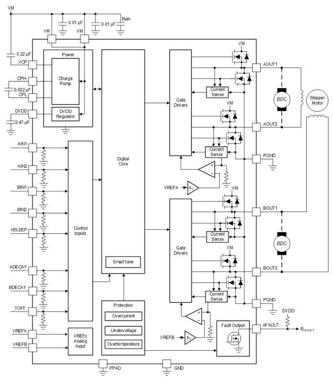
Figure 7-2. DRV8434P Block Diagram
