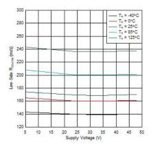
Figure 6-5. Low-Side  $R_{DS(ON)}$  over Supply Voltage
