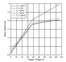
Figure 6-1. Sleep Current over Supply Voltage
