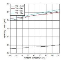
Figure 6-4. Operating Current over Temperature
