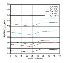
Figure 6-7. High-Side R<sub>DS(ON)</sub> over Supply Voltage
