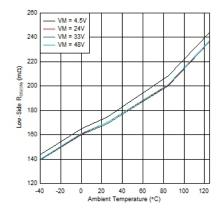
Figure 6-6. Low-Side  $R_{DS(ON)}$  over Temperature
