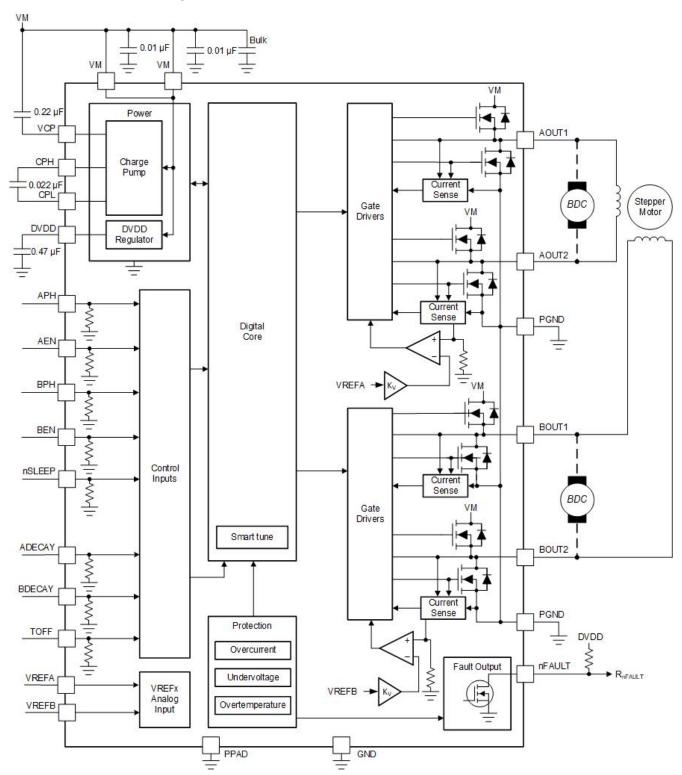
Figure 7-1. DRV8434E Block Diagram
