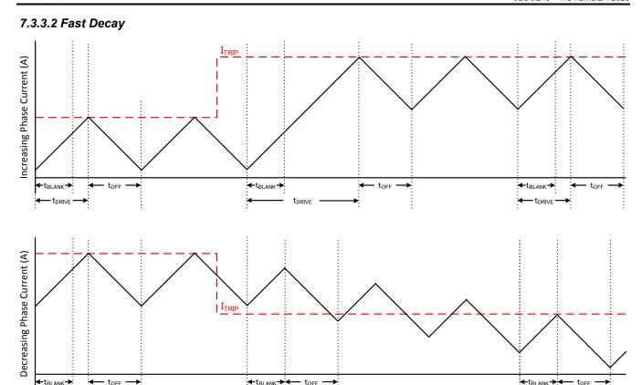
Figure 7-6. Fast/Fast Decay Mode
