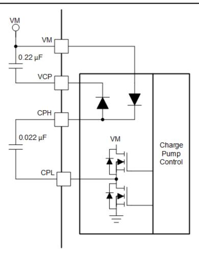
Figure 7-9. Charge Pump Block Diagram
