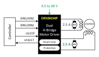
Figure 3-2. DRV8434P Simplified Schematic
