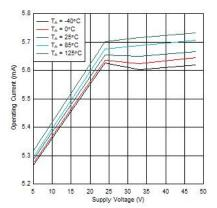
Figure 6-3. Operating Current over Supply Voltage
