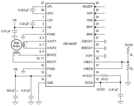
Figure 8-5. Alternate Application Schematic
