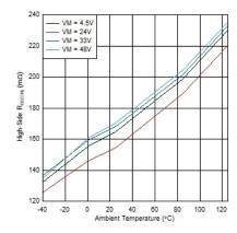
Figure 6-8. High-Side  $R_{DS(ON)}$  over Temperature
