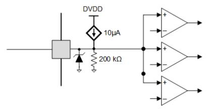
Figure 7-12. Quad-Level Input Pin Diagram
