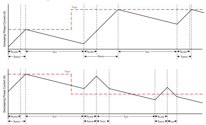
Figure 7-7. Smart tune Dynamic Decay Mode
