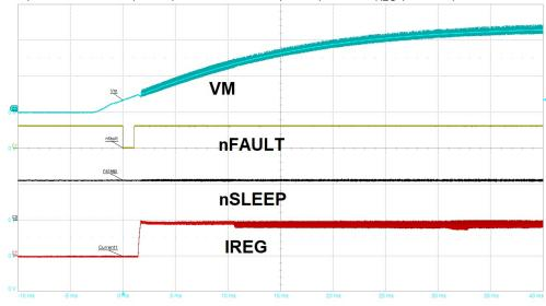
Figure 8-3. Device Power-up with Supply Voltage (VM) Ramp
