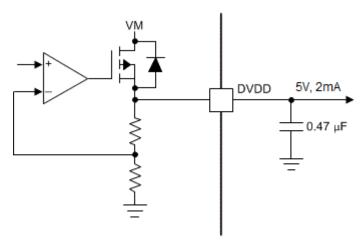
Figure 7-10. Linear Voltage Regulator Block Diagram
