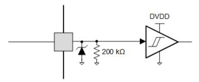
Figure 7-11. Logic-level Input Pin Diagram
