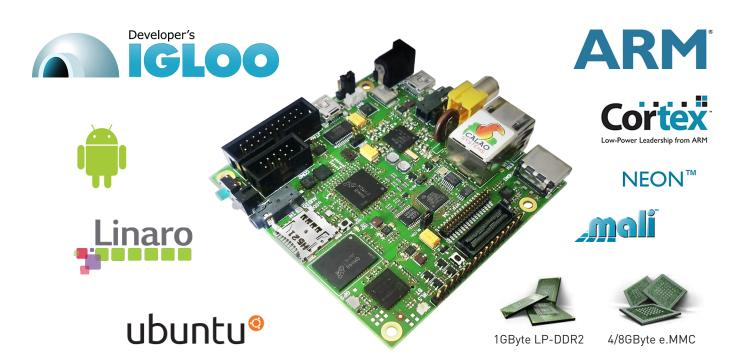
Snowball is a low-power, low-cost single board computer based on the ST-Ericsson Nova™ A9500 processor (Dual Cortex A9 and Mali 400 GPU). Snowball enables hobbyists and professional developers to prototype new embedded designs and applications for Android and Ubuntu.
