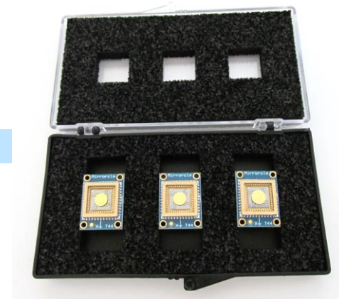
MEMS Mirrors in DK-026 (TINY48.4 connectorized packages)
