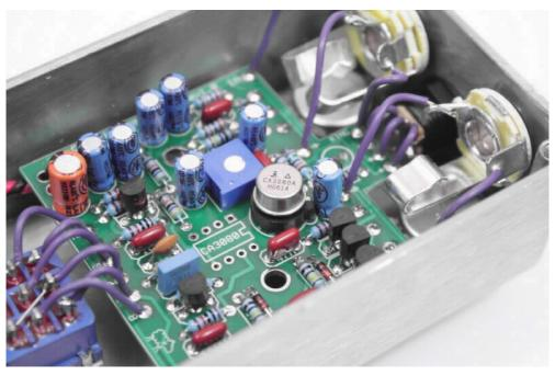
Once you've install the IC, it's time to test the pedal. If you don't get any sound at first, don't worry. You will need probably need to adjust the trimpot. If your trimpot isn't already set at the middle of its rotation, do so. This may or may not be the optimal setting for the trimpot, but it should definitely produce sound and be a good starting point for fine tuning.
