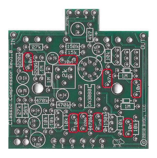
Step 6: Add the film and ceramic disc capacitors. These are not polarized and can be inserted into the PCB either way.
