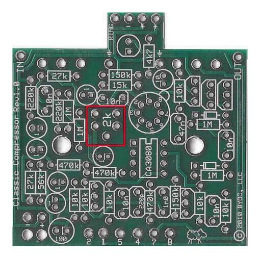
Step 3: Add the trim pot. The space on the PCB has 5 holes, but the trim pot will only have 3 leads. This is so that the PCB can accept a variety of different brands and styles of trim pot. There should only be 1 way that your trim pot will fit into the PCB without having to bend the leads.
