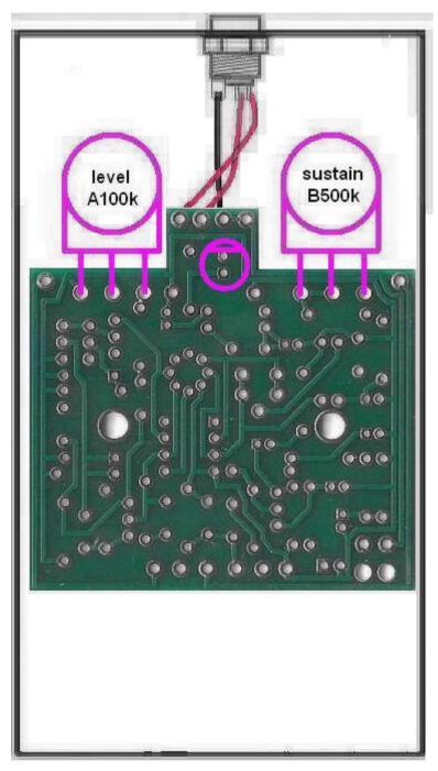
Step 3: Flip the PCB over so that the bottom or solder side is up. Insert the A100k(LEVEL), B500k(SUSTAIN) potentiometers, and the LED into the bottom side of the PCB. DO NOT SOLDER ANYTHING YET!!! The LED will have one lead that is longer than the other. The longer lead goes in the hole with the square solder pad.
