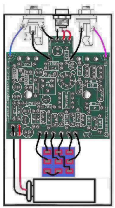
Step 3: Connect the pre stripped and tinned wires to the 1/4" jacks. Step 4:
