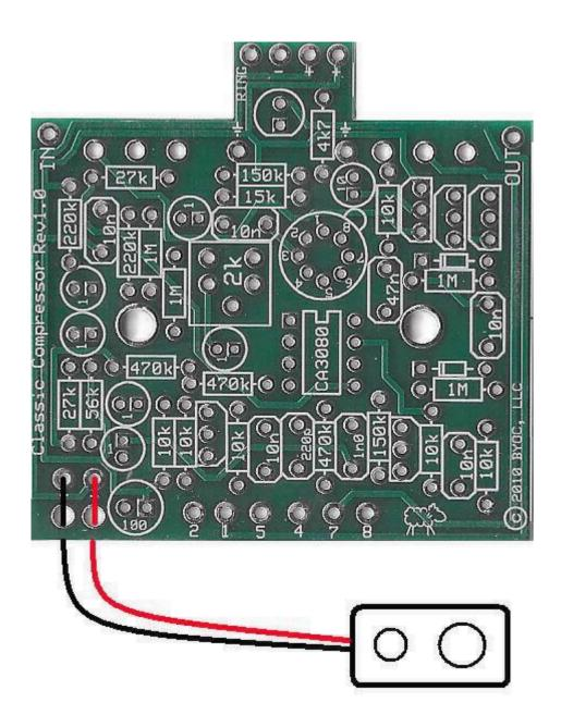
Step 8: Add the battery snap. Thread the solder ends of the battery snap into the strain relief holes from the bottom solderside of the PCB and out through the top. Insert the solder ends of the battery snap wires into the topside of their respective solder pads. Solder on the bottom side of the PCB. Remember the red wire goes in the "+" hole and the black wire goes in the "-" hole.
