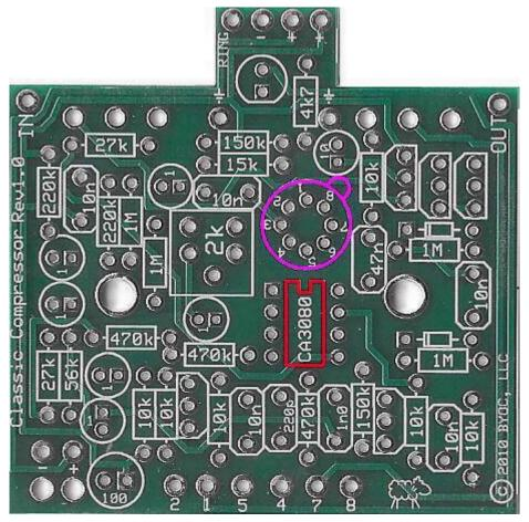
STEP 4: Add the 8 pin IC socket. **ONLY SOLDER THE SOCKET! NOT THE ACTUAL IC!** This is a socket. The socket gets soldered to the PCB. The ICs get inserted into the sockets. The actual IC chip itself, never gets soldered. You will insert the IC into the socket after the entire pedal has been built.
