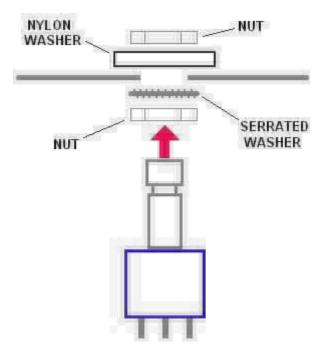
Step 2: Install the footswitch. Orient the footswitch so that the flat sides of the solder lugs are like the diagram below. NOTE: There are no actual number markings on the footswitch. There are two correct ways you can orient the footswitch. They are both 180 degrees of each other. Either way is fine. It does not matter as long as the flat sides of the solder lugs are running horizontal, not vertical.
