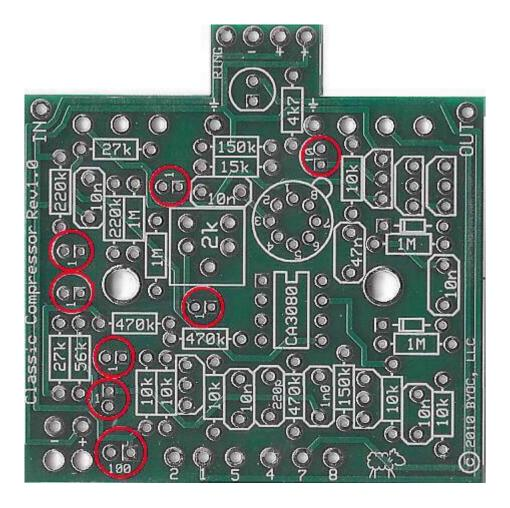
STEP 7: Add the aluminum electrolytic capacitors. These are polarized. The positive end will have a longer lead and should go in the square solder pad. The negative end will have a shorter lead with a black or white stripe running down the body of the capacitor.
