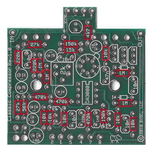
STEP 2: Add the resistors . Resistors are not polarized, so it does not matter which end goes in which solder pad. Take your time and be sure not to confuse similarly banded resistors such as the 470k with the 4k7 or the 10k with the 100k. If you have difficulty reading the color bands, use a digital multimeter to test the value of each resistor.
