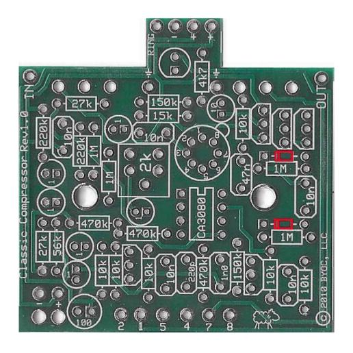
STEP 1: Add the diodes. Be sure to match the end of the diode with the stripe to the layout on the PCB. The stripped end should go in the square solder pad.
