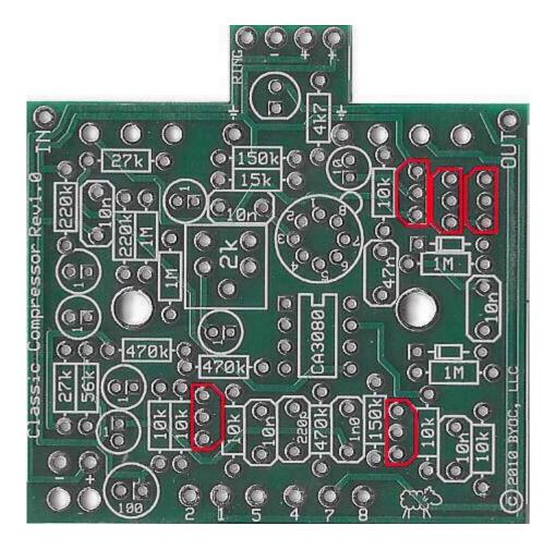
Step 5: Add the Transistors. Be sure to orient the transistors so that the flat side of the tansistor body matches up with the flat side on the PCB layout. This is the same for both the 2N5088 and 2SC1849 or any transistor that is supplied with this kit.
