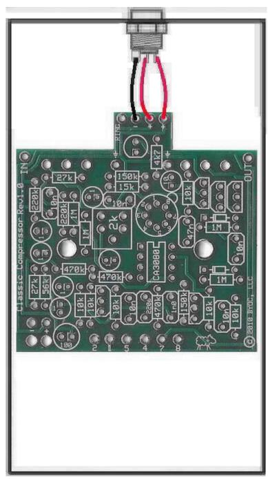
**Step 2:** Connect the TIP (negative) terminal of the DC adaptor jack to the "-" eyelet on the PCB with 2 inches of hook up wire. Connect the SLEEVE of the DC adaptor jack to the "+" eyelet on the far right side of the PCB with 2 inches of hook up wire. Connect the battery disconnect terminal of the DC adaptor jack to the "+" eyelet more towards the center of the PCB with 2" of hookup wire. Load the wires in from the bottom of the PCB and solder on the topside.
