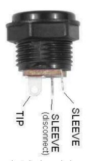
Step 1: Mount the DC adapter jack to the enclosure.
