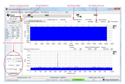
Figure 5. HSDC Pro GUI Main Panel
