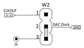
Figure 7. External Clock Signal
