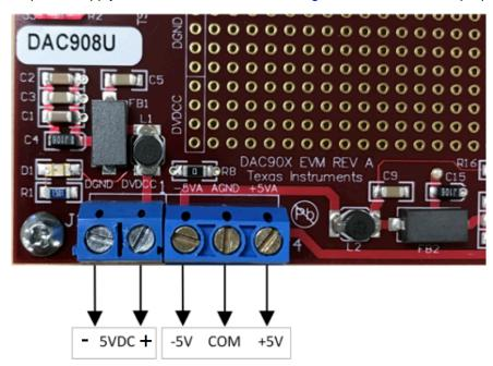
**Figure 4. Power Supply Connections**
