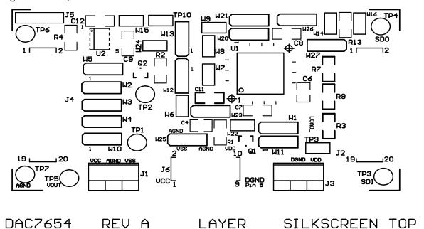
Figure 2–2. Layer 1 (Top Signal Plane)
