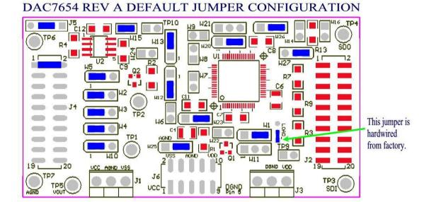
Figure 3–1. DAC7654 EVM Default Jumper Setting
