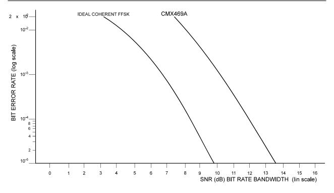
Figure 8 Typical Rx Bit Error Rate vs Signal-to-Noise Ratio
