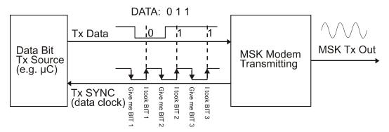
Figure 4 Synchronous Transmit Operation
