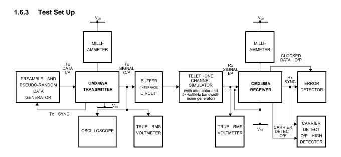
Figure 3 Suggested CMX469A Test Set-Up
