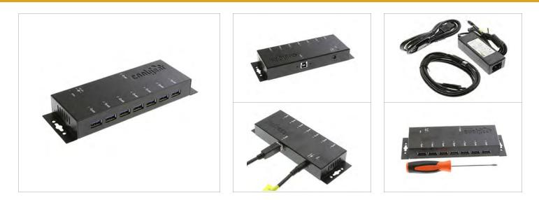
The CG-7U3DS is a 7-Port USB 3.0 Hub that complies with the Universal Serial Bus 3.0 (USB 3.0) Specifications Revision 1.0 and performs at up to 5Gbps Super-Speed. The Hub is DIN-Rail mountable and supports DC-Jack for +12V DC power input. With built-in RISC-like USB 3.0 controller chips, it is backward compatible either when any one of the downstream port is connected to a USB 1.1 or USB 2.0 compliant device, or when the upstream port is connected to a USB 1.1 or USB 3.0 compliant host.
