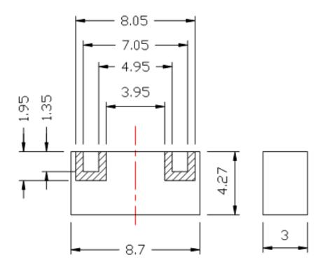
Dimensions in mm Tolerance : ±0.25
