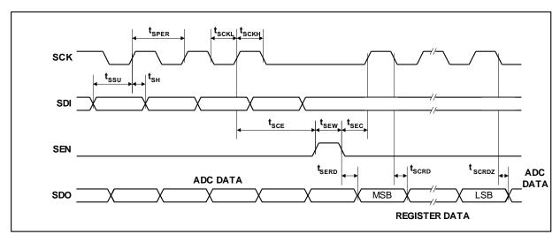
Figure 3 Serial Interface Timing
