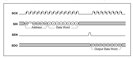
Figure 16 Serial Interface Register Read-back
