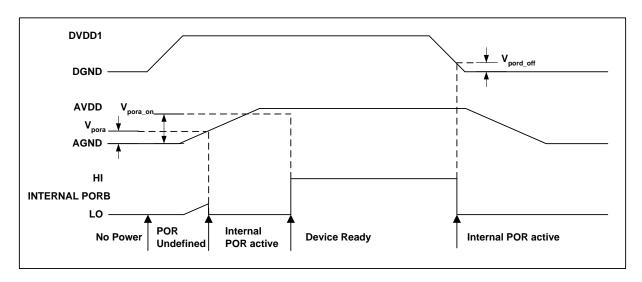
Figure 6 Typical Power up Sequence where DVDD1 is Powered before AVDD
