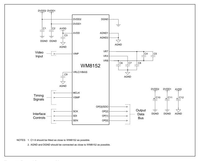
Figure 22 External Components Diagram
