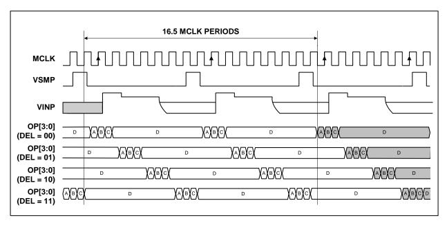
Figure 21 Mode 4 Operation (MCLK:VSMP Ratio = 8:1)
