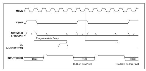
Figure 8 Relationship of RLCINT, MCLK and VSMP to Internal Clamp Pulse, CL
