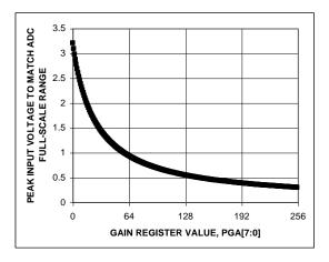
Figure 10 PGA Gain Characteristic
