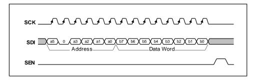
Figure 15 Serial Interface Register Write
