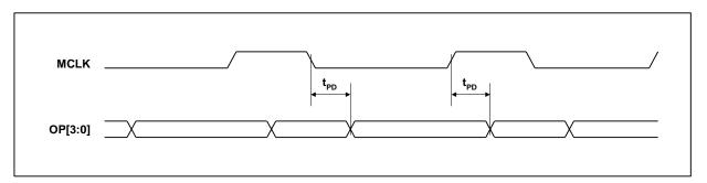
Figure 2 Output Data Timing
