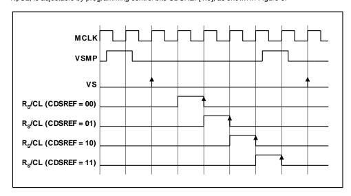
Figure 9 Reset Sample and Clamp Timing
