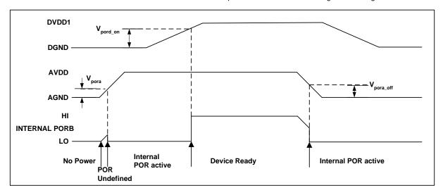
Figure 5 Typical Power up Sequence where AVDD is Powered before DVDD1
