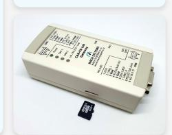
The gateway can be powered externally via a DSUB connector or via a micro-USB connector. LIN bus requires external power. All ground signals are connected.
